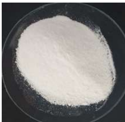
Figure 24: Appearance of the KC-Bioactive particles produced by the DS method with spray-drying
