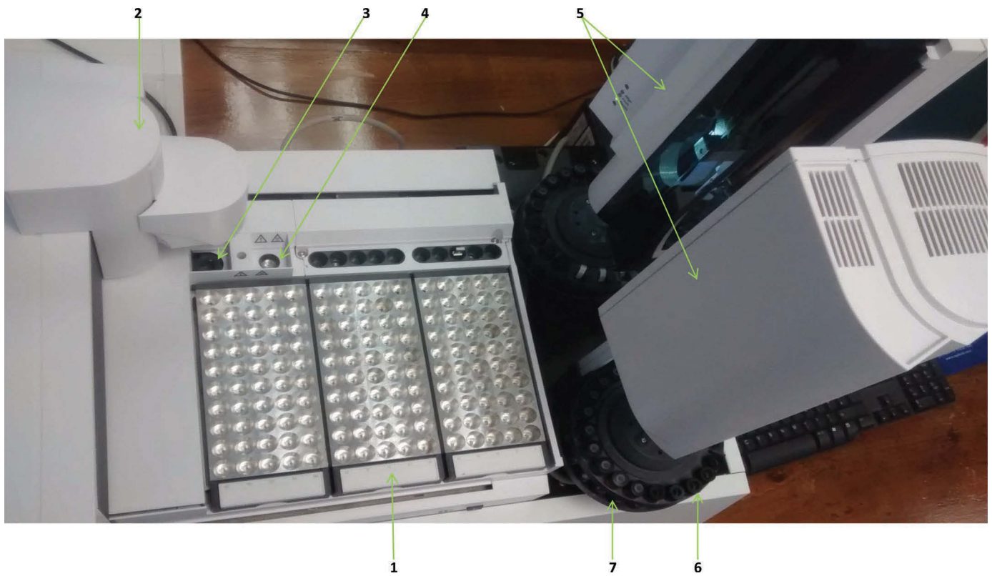
Figure 1. Schematic of Agilent Sample Prep Workbench System (Agilent Technologies Ireland Ltd., Little Island, Cork, Ireland). 1 = sample trays; 2 = robotic arm; 3 = vial vortex; 4 = vial heater; 5 = auto-sampler towers; 6 = waste vials; 7 = solvent wash vials.
