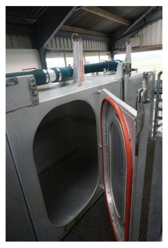
Figure 1. Portable accumulation chamber.
