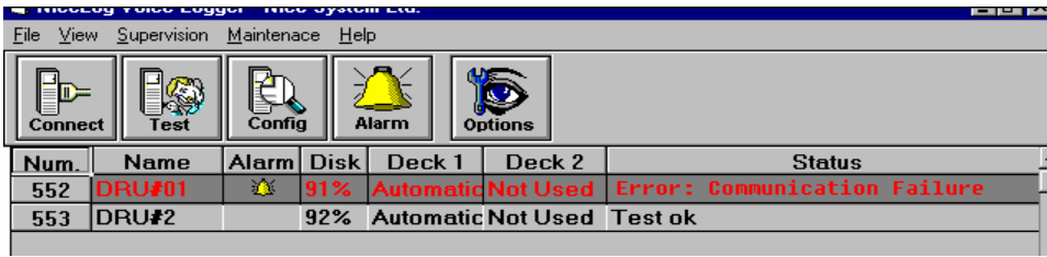
Figure 7. DVRS screen showing an alarm.
