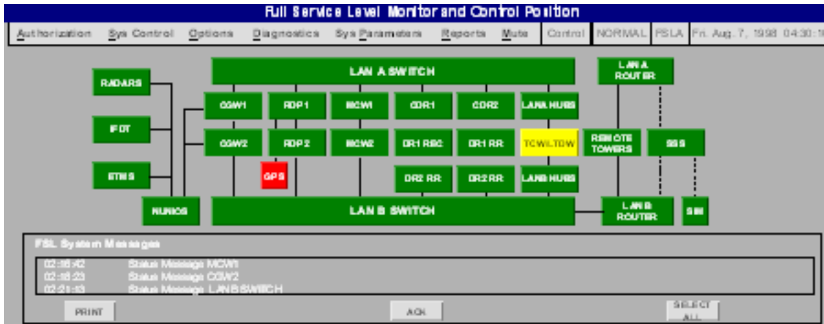
Figure 2. TO system display showing primary status area (colored rectangles) and secondary area (white text below primary status area).
