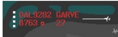
Figure 18. Data block of an aircraft that violated the D-Taxi clearance.
