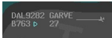
Figure 13. Data link indicator in a data block showing that the participant sent the D-Taxi clearance to the aircraft.
