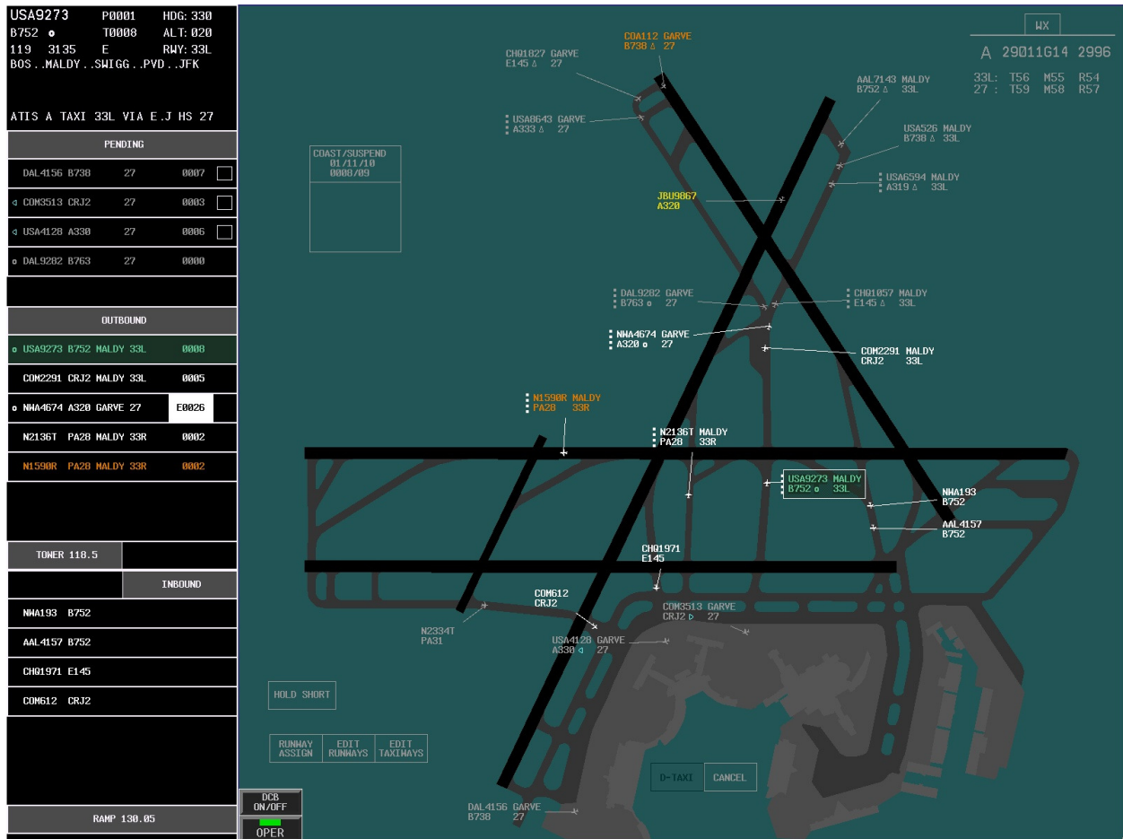
Figure 2. Screenshot of the ground control position.
