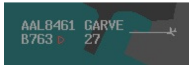
Figure 15. Data link indicator showing a failed data link transmission.
