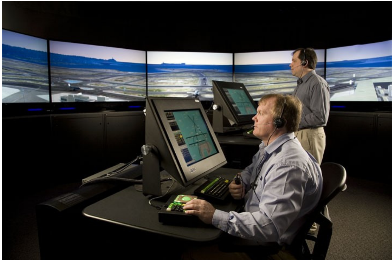
Figure 1. The experiment apparatus including the ground (foreground) and local (background) control positions and the OTW view. The STARS display (not shown) was located to the right of the local controller.
