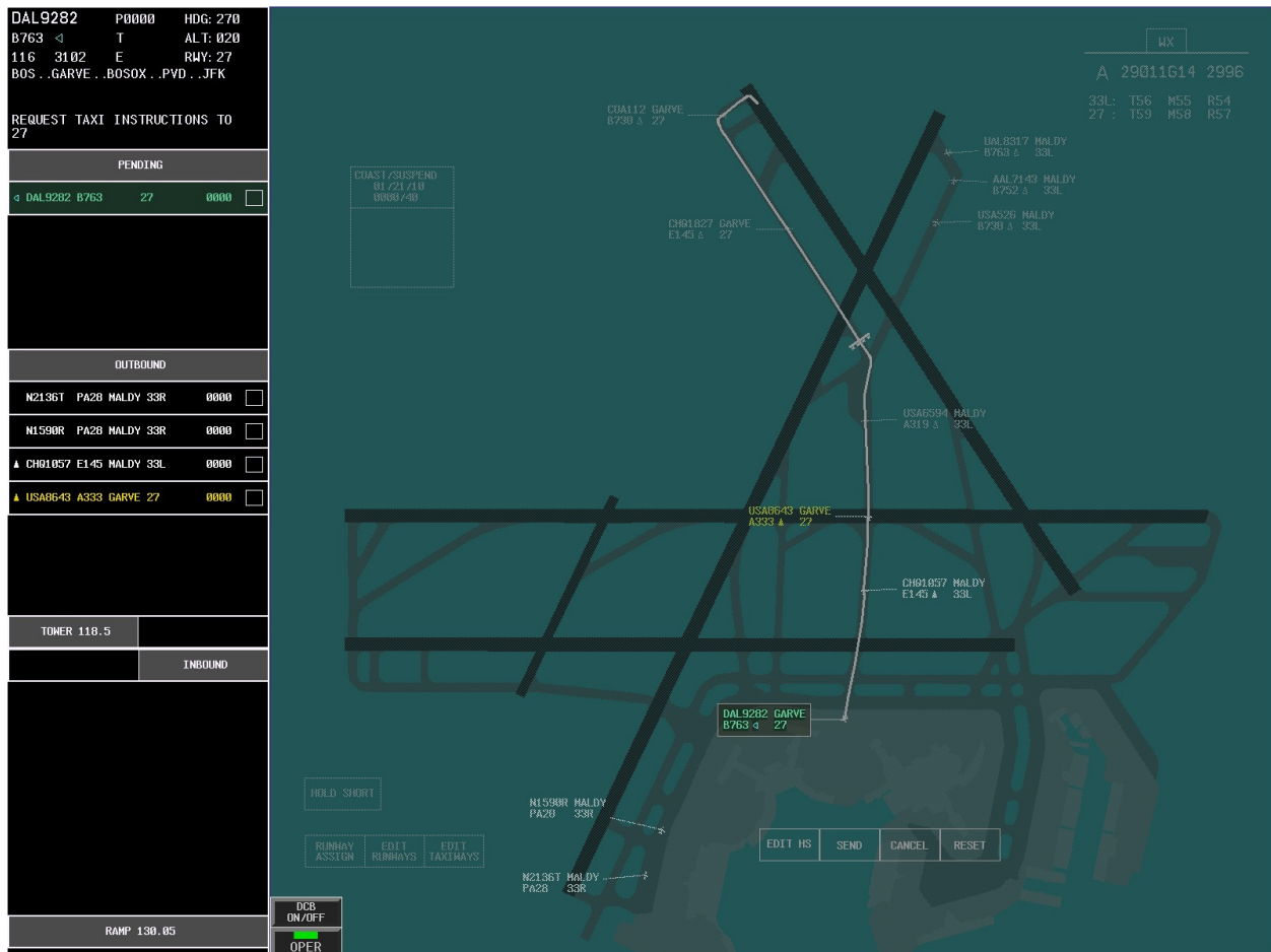
Figure 9. The ground control position in the D-Taxi construction mode.
