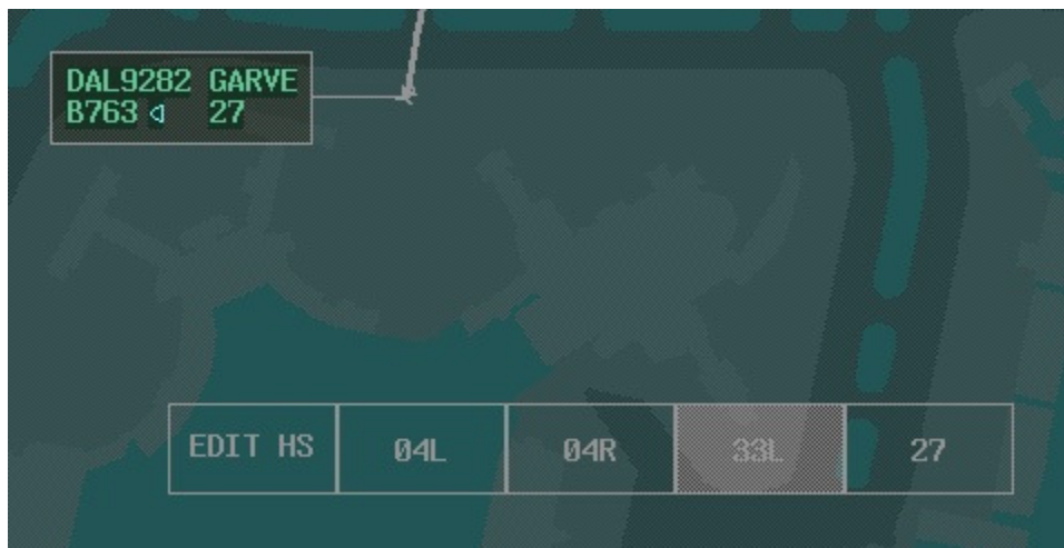
Figure 11. Selected data block and edit buttons for adding or removing a hold short point.
