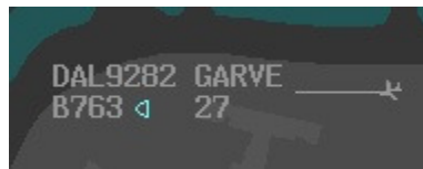
Figure 5. Data link indicator indicating a pilot request for taxi instructions.
