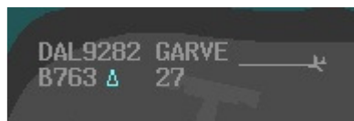
Figure 8. Data link indicator for a deferred data link request.
