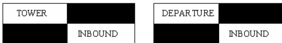
Figure 18. Recommended button/header design for the ground (left) and local (right) control positions to prevent inadvertent selection of a proximal button.
