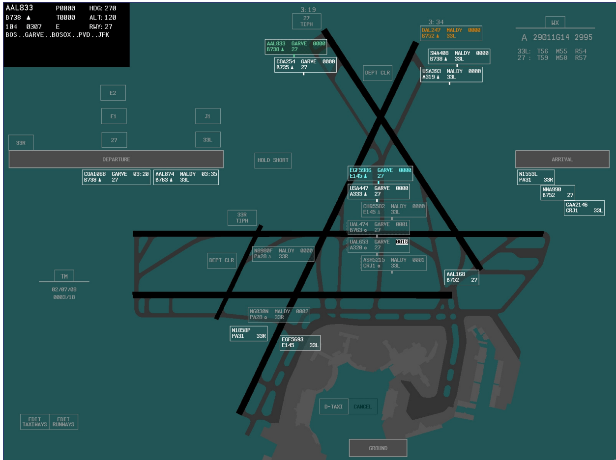
Figure 4. The PS-TODDS interface for the local control position.
