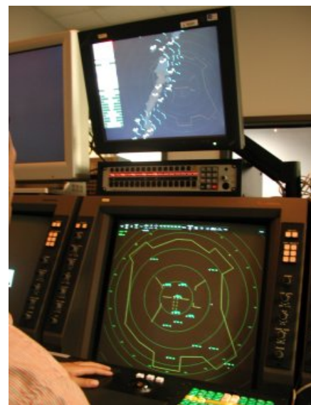
Figure 8b. Advanced weather information presented on the WIDS (top display) and traffic data on the TCW (bottom display).
