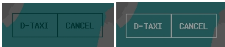
Figure 35. Inactive (left) and active (right) D-Taxi and Cancel buttons on the TODDS.
