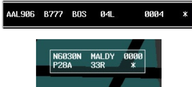
Figure 9. The Flight Data Amendment indicator on an FDE in the Integrated (top) and P-S (bottom) EFDIs.
