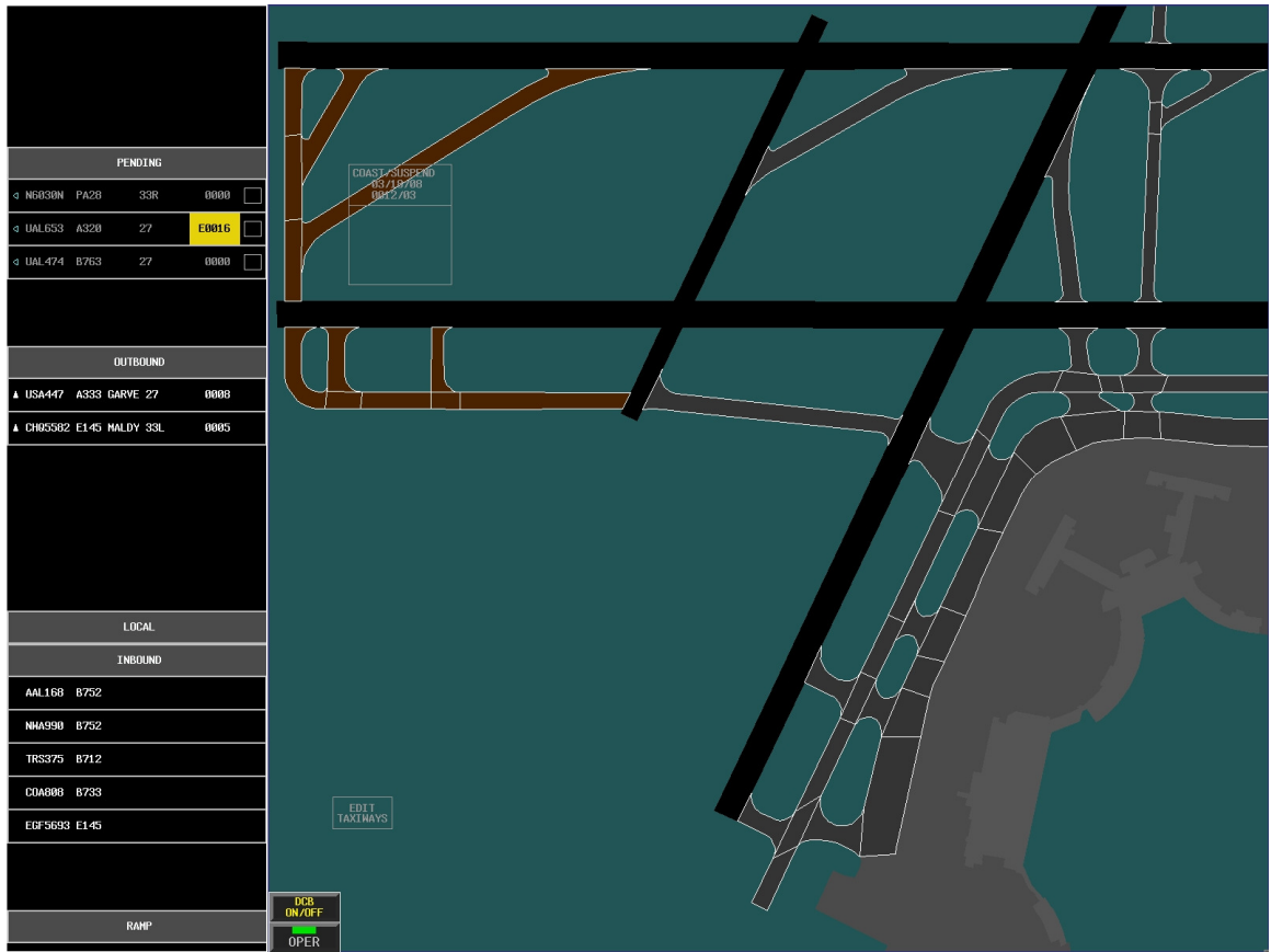
Figure 29. Selected closed taxiway segment indicators in the zoomed editing view of the Integrated TODDS.
