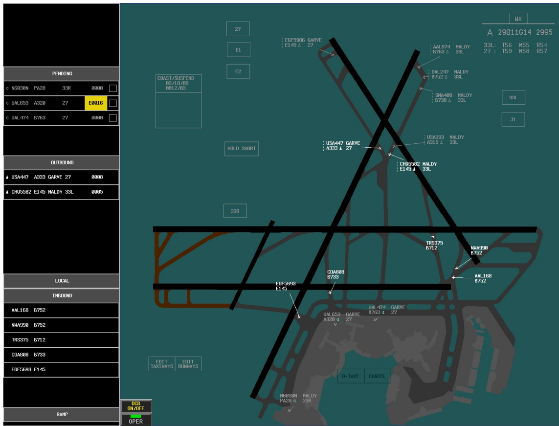
Figure 30. The closed taxiway segment indicators on the Integrated TODDS.
