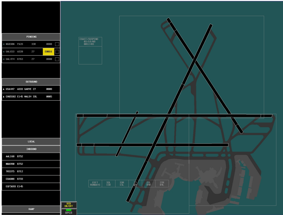
Figure 25. The closed runway edit screen including airport sectors and buttons in the Integrated TODDS.
