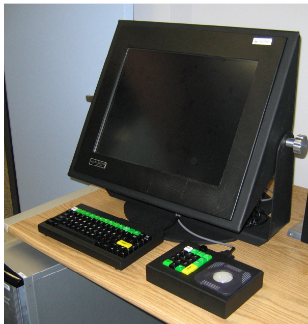
Figure 1. Hardware used to implement the prototype displays including resistive touch display, display mount, keyboard, and trackball/keypad.
