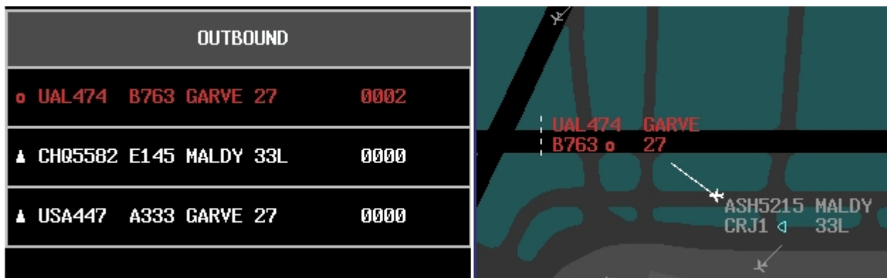
Figure 40. An FDE and data block highlighted in red, indicating that the aircraft is not conforming to the D-Taxi clearance.
