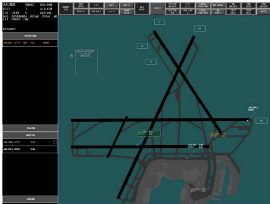
Figure 3. The primary elements of the local controller's Integrated display including the surface situation display, electronic flight data lists, and readout area.
