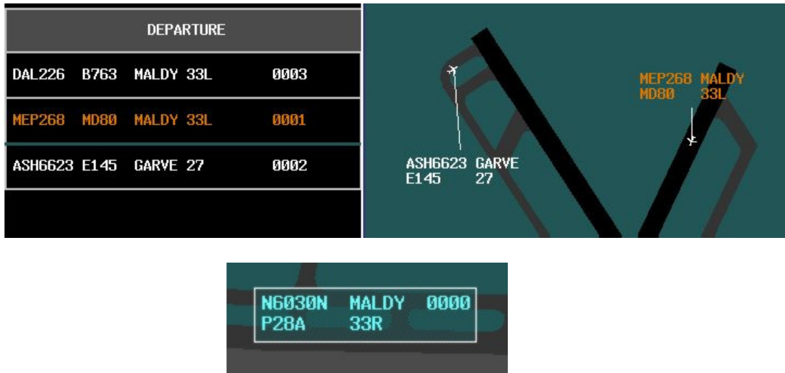
Figure 14. A highlighted aircraft in the Integrated EFDI (top) and a selected and highlighted FDE in the P-S EFDI (bottom) retains ownership information.
