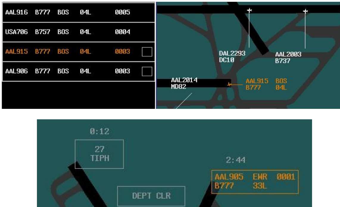
Figure 13. A highlighted aircraft in the Integrated (top) and P-S EFDI (bottom) loses ownership information.
