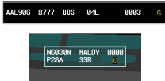
Figure 6. The expired aircraft specific timer icon on an FDE in the Integrated (top) and P-S (bottom) EFDIs.
