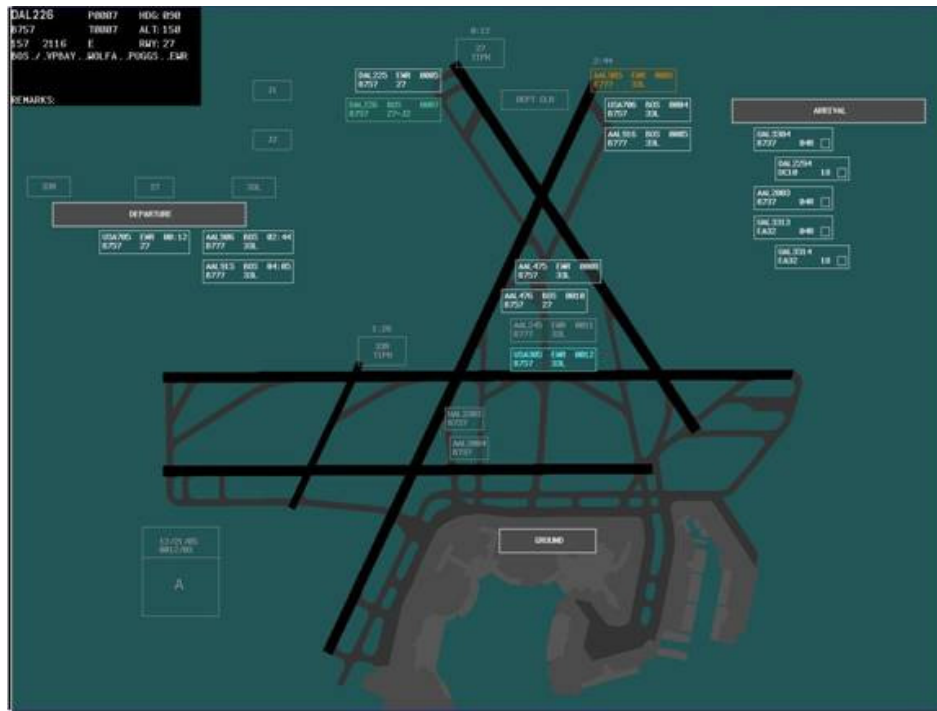
Figure 4. The primary elements of the Perceptual-Spatial display including flight data elements, the readout area, buttons, and system information window.
