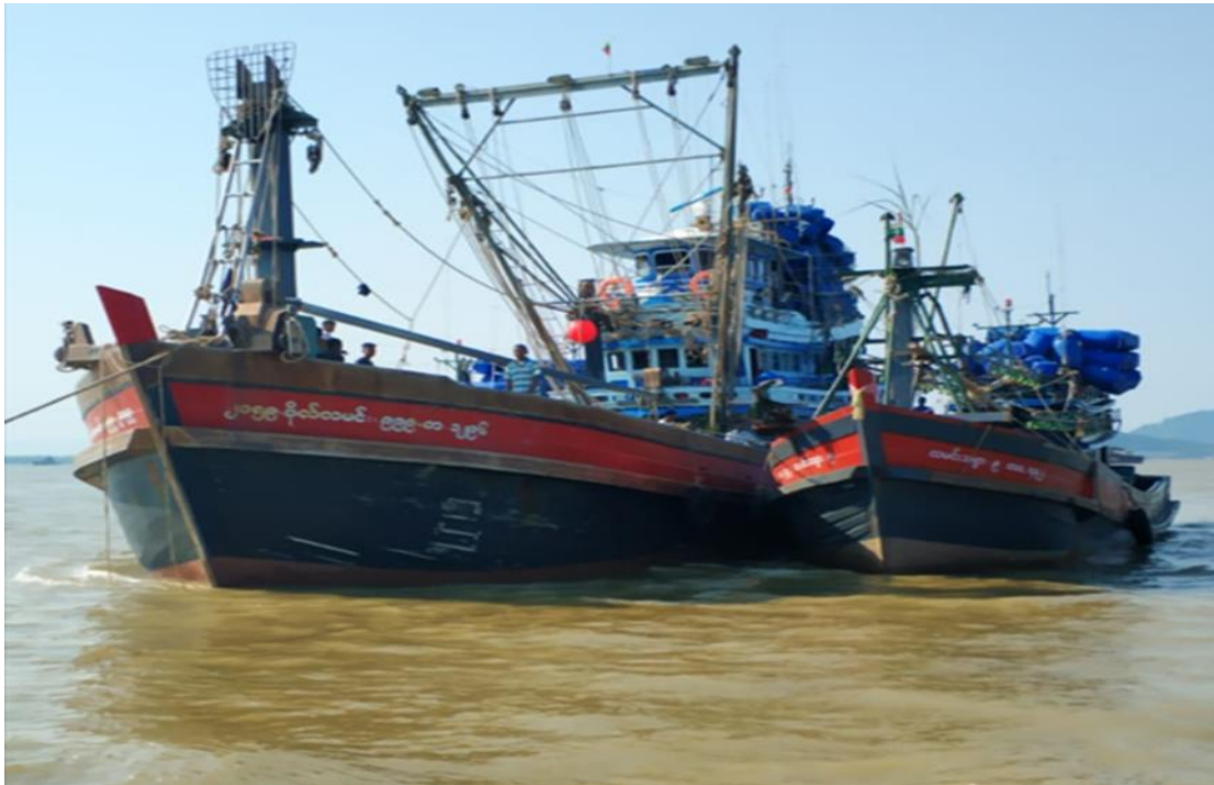
Figure 4. Purse seine vessel (left) and light luring vessel (right) in Myeik offshore fisheries
