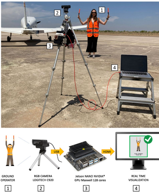
Fig. 5 General description of the test setup used in the course of this work
