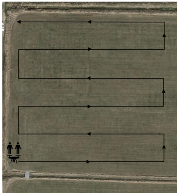
Figure 21. Visual depiction of the parallel line search that is inputted by the UAV Pilot to navigate the UAV within a search region
