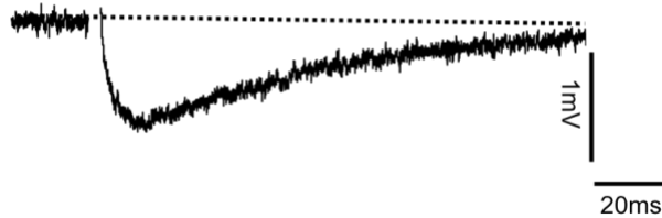
Figure 2.4. NMDAR mediated fEPSP amplitude response. This illustration is an example measurement of NMDAR response amplitude. The NMDAR-mediated component was obtained after 10 \mu M NBQX, 50 \mu M PTX, and 1 \mu M CGP55845, were added to the perfusate in order to block AMPAR, GABA A and GABA B mediated transmission, respectively. Subsequently, the stimulus intensity was increased by 100-150% to obtain the measurement of NMDAR-fEPSP response amplitude.
