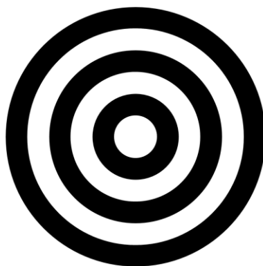
Figure 7: A typical Bessel beam profile. The white regions (indicating laser beam) show negligible diffraction over the working range of a microscope, meaning they can be used over longer distances than a normal Gaussian trap.
