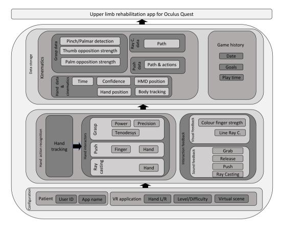
Fig. 1. Multi-layer architecture that supports RI for the development of virtual upper-limb rehabilitation applications.
