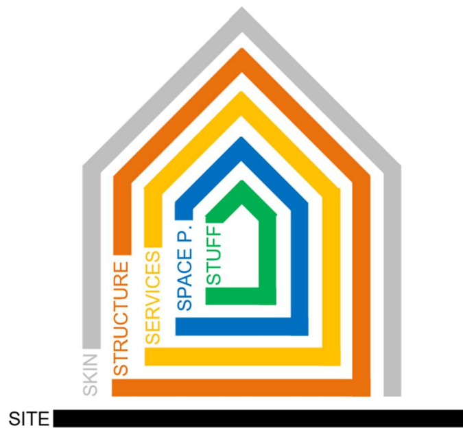
Figure 3: Brand's (1994) shearing layer concept that divides a building into several layers, which have a somewhat common aggregated lifetime (own image).
