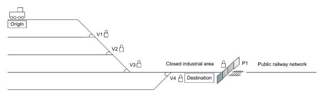
Figure 21. The AutoCar has a static local permit for operation in a closed industrial area.
