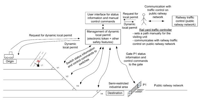
Figure 22. The AutoCar has a dynamic local permit for operation in a semi-restricted industrial area.
