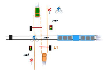
Figure 10. A level crossing with traffic lights and level crossing safety system.
