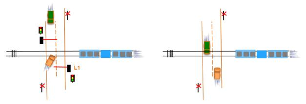
Figure 12. A level crossing with and without traffic lights and level crossing safety system.
