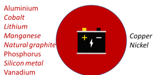
Figure 9. Raw material needs in stationary battery applications. Red colour = critical raw materials. Italics = strategic raw materials.
