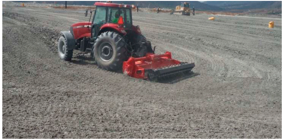
Figure 17. Filtered tailings moved by a plow with nine 24-inch discs to aerate the cake.
