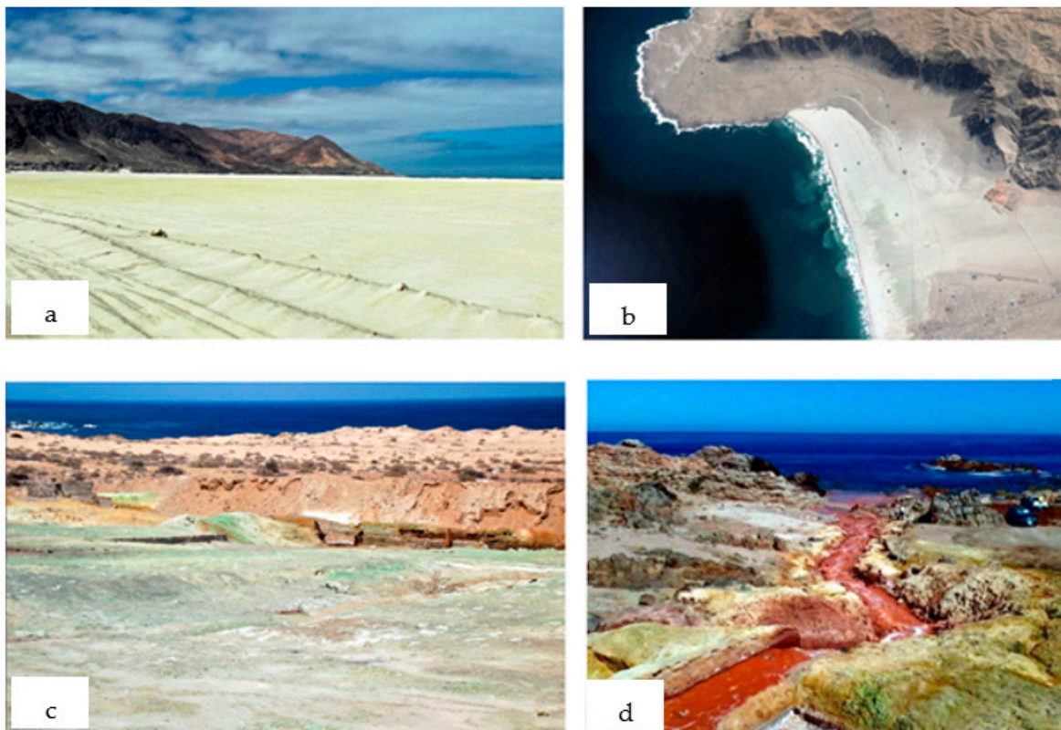
Figure 6. Mine tailings disposal in Chañaral Bay, Chile—Discharge of mine tailings to Salado River and final disposal in the sea. (a) Panoramic view of mine tailings beach in Chañaral Bay, (b) aerial view of Chañaral Bay with mine tailings, (c) mine tailings with oxidation, and (d) discharge point of mine tailings and process water to Caleta Palitos Bay.
