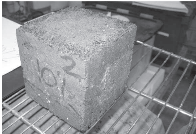
Plate 4: 10% Rubber sample at 50 freeze/thaw cycles
