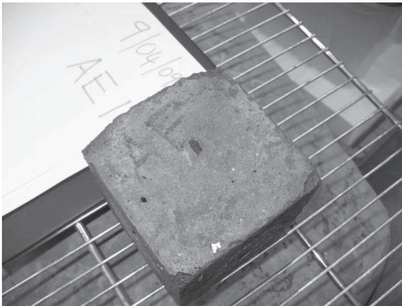
Plate 2: Air Entrained sample at 50 freeze/thaw cycles
