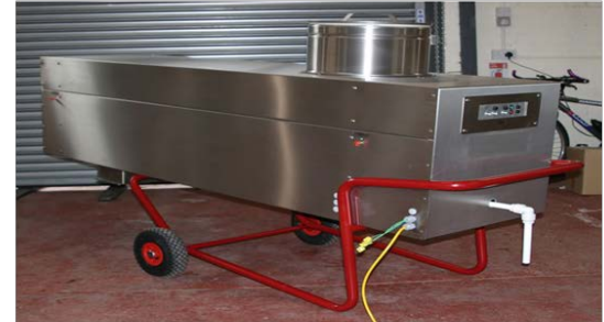
Commercial macerator connected to industrial composting chambers
