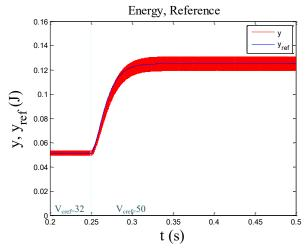
Fig. 11. Variations of the energy stored in the capacitor and its reference with respect to time when the output reference voltage changes at  $t=0.25\ s$
