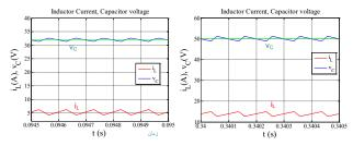
Fig. 10. Variations of the capacitor voltage with respect to time when the output reference voltage changes at  $t=0.25\ \rm s$
