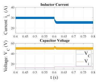
Fig. 19. Inductor current and capacitor voltage for an input voltage variation
