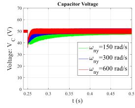
Fig. 22. Capacitor voltage waveforms when the load resistance is reduced at t = 0.25 s for different control parameters of the inner and outer loop
