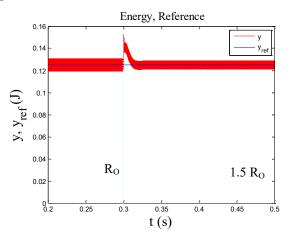
Fig. 17. Energy stored in the capacitor and its reference when the load resistance is increased by 50%
