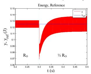
Fig. 13. Energy stored in the capacitor and its reference when the load resistance is halved at  $t=0.3\ s$
