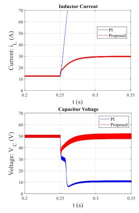
Fig. 26. Inductor current and capacitor voltage for a variation of inductance 180% of its nominal value
