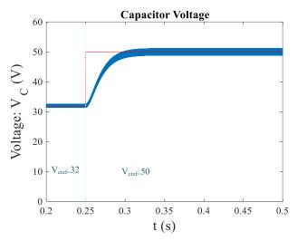
Fig. 9. Variations of the capacitor voltage with respect to time when the output reference voltage changes at t = 0.25 s
