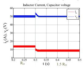
Fig. 16. Inductor current and capacitor voltage for a 50% increase in the load resistance at  $t=0.3\ s$
