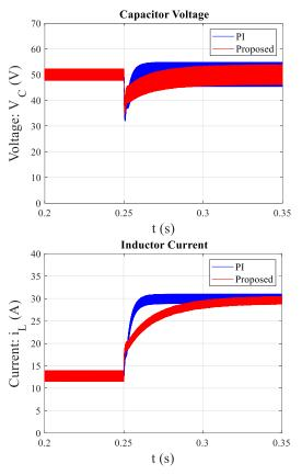
Fig. 27. Inductor current and capacitor voltage for a variation of capacitance -50% of its nominal value
