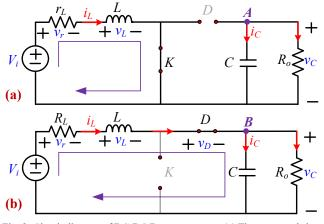
Fig. 2. Circuit diagram of DC-DC Boost converter: (a) The command signal is one, (b) The command signal is zero
