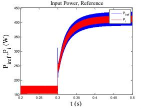
Fig. 15. Variations of the input power and its reference when the load resistance is halved at  $t\,{=}\,0.3~{\rm s}$
