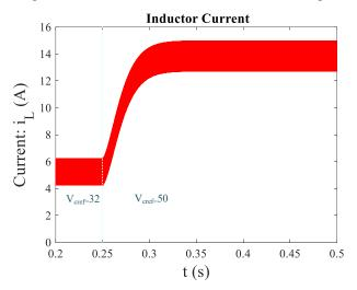
Fig. 8. Variations of the inductor current with respect to time when the output reference voltage changes at t = 0.25 s
