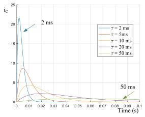
Fig. 5. Capacitor current response with step input for different time constant  $\tau$
