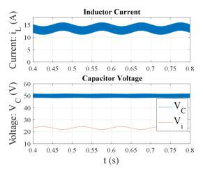
Fig. 20. Inductor current and capacitor voltage for a variation of input voltage with a sinusoidal waveform
