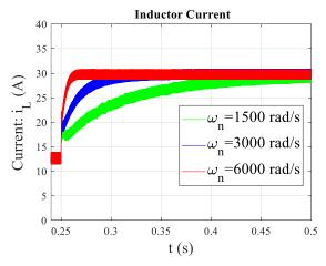
Fig. 21. Inductor current waveforms when the load resistance is reduced at t = 0.25 s for different control parameters of the inner and outer loop
