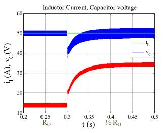
Fig. 14. Inductor current and capacitor voltage when the load resistance is halved at  $t\,{=}\,0.3~{\rm s}$
