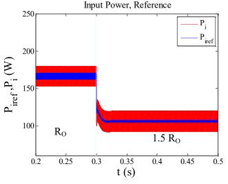
Fig. 18. Variations of the input power and its reference when the load resistance is increased by 50%
