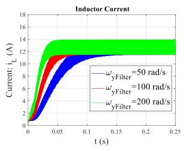
Fig. 23. Inductor current waveforms during startup when cutoff frequency of the energy filter  $\omega_{yFilter}$  is varied
