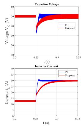
Fig. 25. Inductor current and capacitor voltage for a variation of inductance 100% of its nominal value
