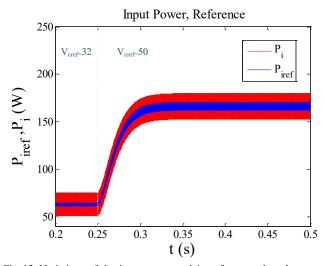
Fig. 12. Variations of the input power and its reference when the output reference voltage changes at  $t\,{=}\,0.25~{\rm s}$
