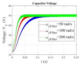
Fig. 24. Capacitor voltage waveforms during startup when cutoff frequency  $\omega_{yFilter}$  of the energy filter is varied
