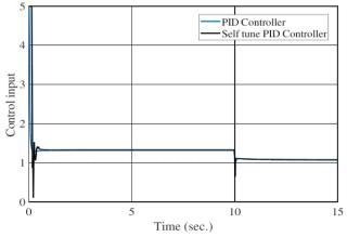
Fig. 15. Controller output for PID and fuzzy self-tuning of PID
