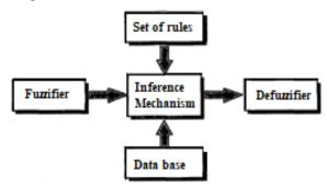
Fig. 4. Block diagram of the fuzzy-logic controller
