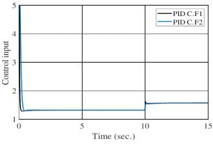
Fig. 13. Controller output for PID C.F1 and PID C.F2
