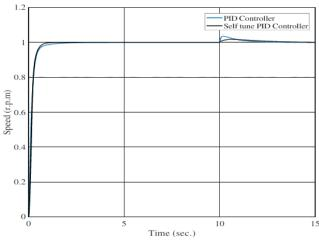
Fig. 14. DC servo motor system response with PID and self-tuning of PID
