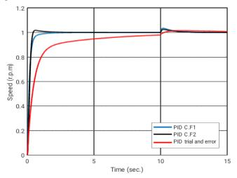
Fig. 10. DC servo motor system response with PID C.F1, PID C.F2 and trial and error-PID controllers
