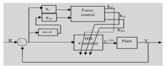
Fig. 5. Fuzzy self-tuned pid controller
