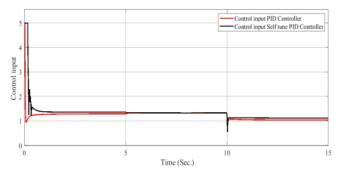
Fig. 17. Controller output for PID and "fuzzy self-tuning PID"
