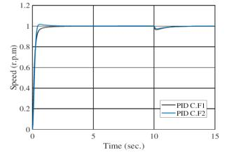
Fig. 12. DC servo motor system response with PID C.F1 and PID C.F2
