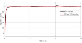
Fig. 16. DC servo motor system response with PID and self-tuning of PID
