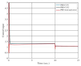
Fig. 11. Controller output for PID C.F1, PID C.F2 and trial and error-PID controllers
