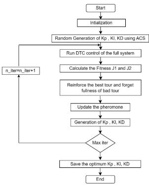
Fig. 3. Flowchart of PID controller optimization by ACS
