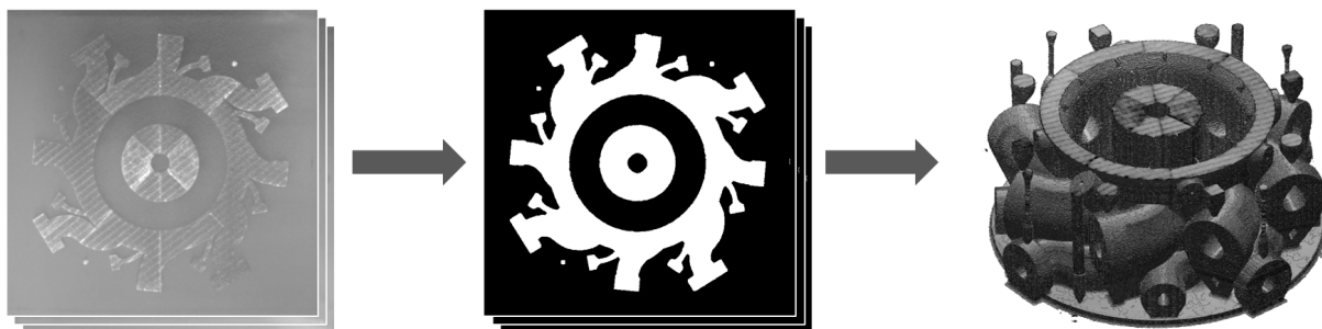
Figure 4: Additive manufacturing reconstruction workflow: from raw images to binary masks to textured voxel model. Data courtesy Additive Industries B.V.
