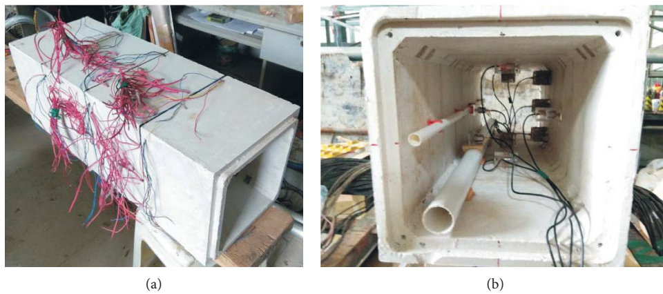
FIGURE 3: Model structure: (a) prefabricated utility tunnel model; (b) pipeline model hold by the tunnel.
