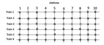
Fig. 2 The stop-skip pattern for trains running on Line 5
