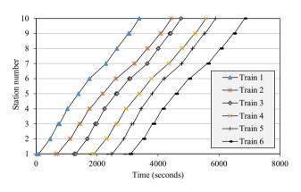
Fig. 5 The time-station graph of the train movement
