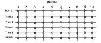
Fig. 4 The skip-stop schedule obtained for the robust optimization model  $% \left( {{{\left[ {{{{\bf{n}}_{{\rm{s}}}}} \right]}_{{{\rm{s}}_{{\rm{s}}}}}} \right)$
