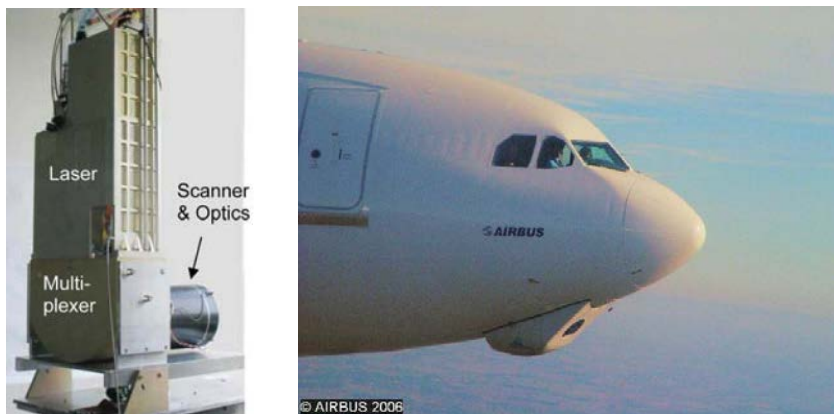
Figure 65: The EADS UV LiDAR developed within the AWIATOR project (left) and the integration in an A340 aircraft during Airbus flight tests (right); the LiDAR is included in the fairing beneath the cockpit
