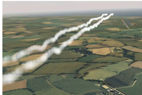
Figure 88: Wake vortex visualisation in the visual system of a flight simulator; from (Spence et al. 2005).
