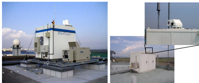
Figure 59: (from left to right) US Lockheed 1.6 & 2 micron Lidars, Japanese Mitsubishi 1.5 micron LiDAR
