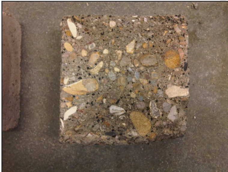
Figure 11 – Rubber particle distribution
