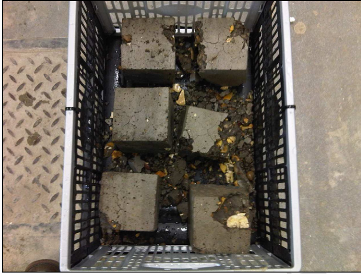
Figure 9 – Batch C (plain) final extent of cube degradation
