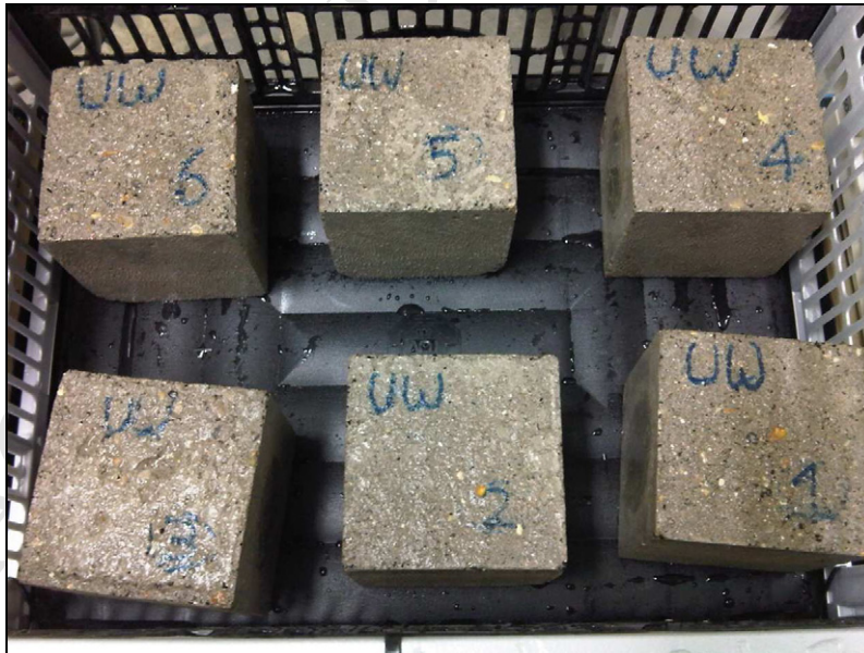
Figure 10 – Batch B (unwashed rubber) final extent of scaling
