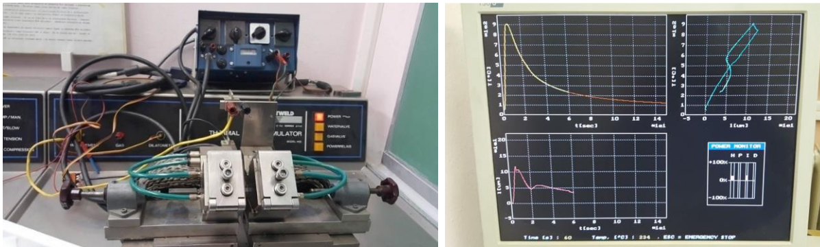
Figure 3. 3 a) Welding simulator and b) real heat treatment diagram (WTCS)
