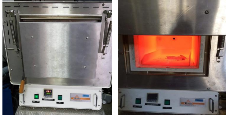
Figure 3.4 Furnace for heat treatment of the specimens
