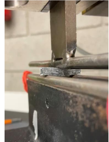
Figure 5. ILSS PLA-SSF testing
