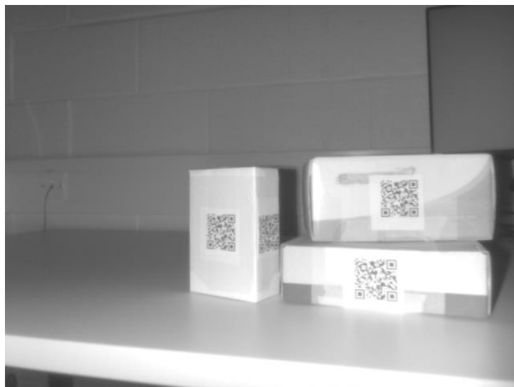
Figure 5: Example of QR code markers to indicate plane centroid position.
