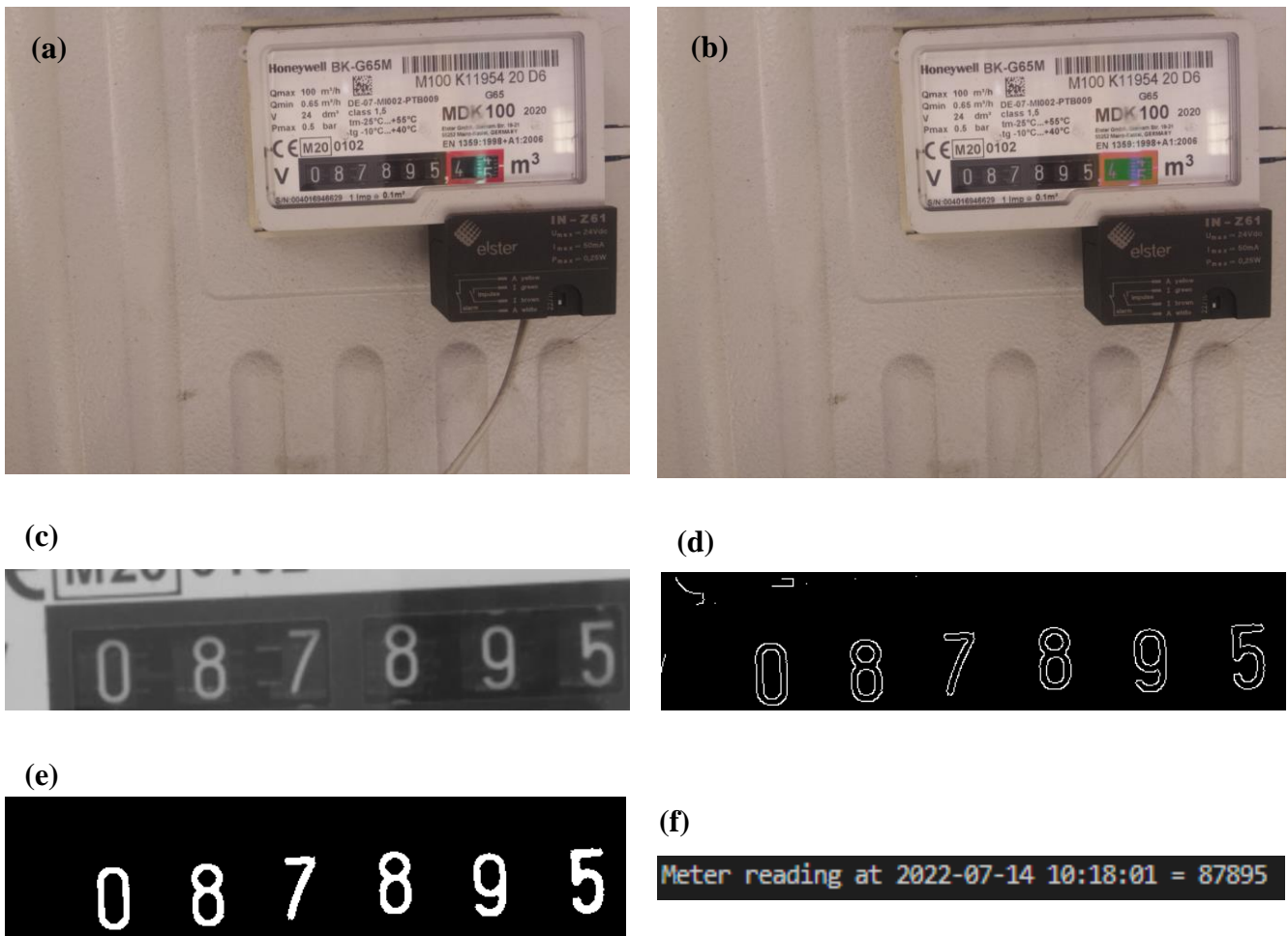
Figure 4. (a) Raw image. (b) Red datum area highlighted. (c) Area of interest cropped. (d) Edges detected. (e) Closed edges filled in. (f) Numbers recognised.
