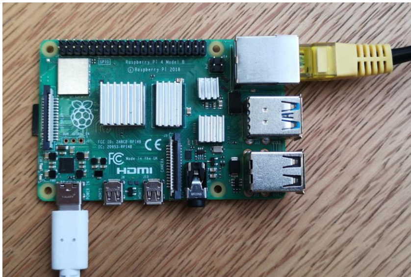
Figure 3. Raspberry Pi model 4B with power and ethernet connections.
