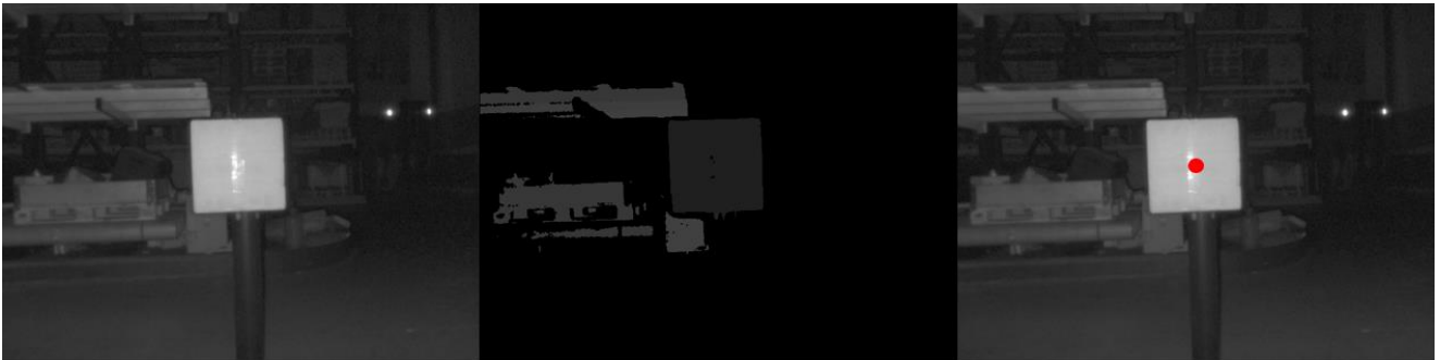
Figure 4: OOI placed on a matt pole (left), Depth image of OOI for Point cloud analysis (centre), OOI with calculated centroid position marked (right).
