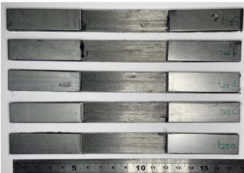
Figure 8. S35 PLA-SSF prepared tensile sample set of five samples
