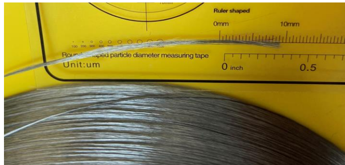
Figure 2. Stainless steel fibre bundle, 90 fibres
