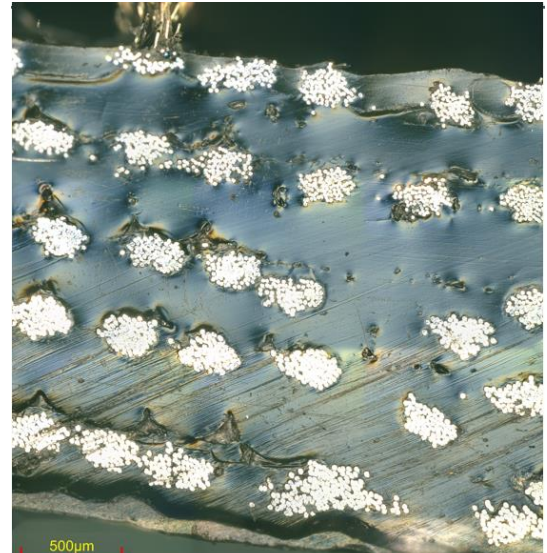
Figure 9. PLA-SSF 3D printed L41 tensile sample cross-section, Olympus DSX1000 microscope
