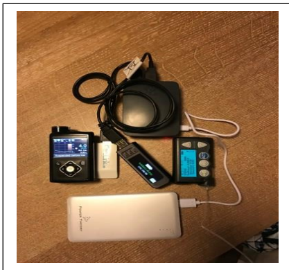
Image 2 Hybrid closed loop consisting of Raspberry Pi, Carelink stick and MiniMed 640g (source: Tim Street, Diabettech.com)
