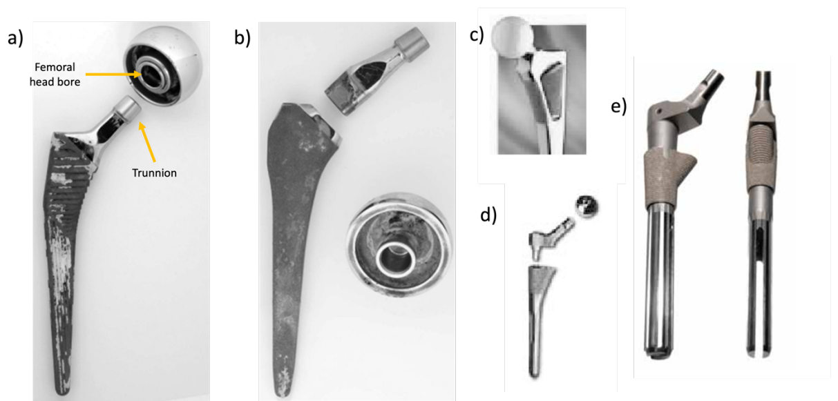
Figure 2.2. Modular femoral components of a THR with a head-neck junction (a), and neck-stem junctions (b), femoral pads (c), proximal shoulders (d), and stem sleeves (e) adapted from (Krishnan et al., 2013; McTighe et al., 2015a).
