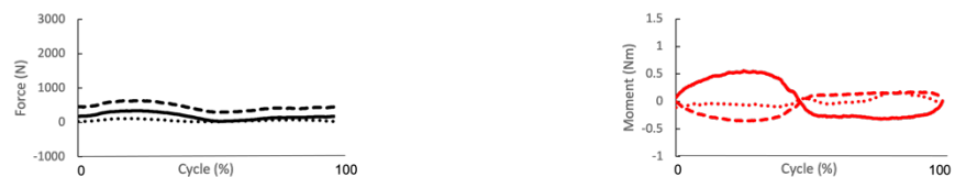
Figure 3.7. Forces and frictional moments representative of daily activities, for (a) walking, (b) stairs up, (c) jogging, (d) sit-to-stand and (e) cycling applied to the base of the trunnion; adapted from (Bergmann et al., 2016).
