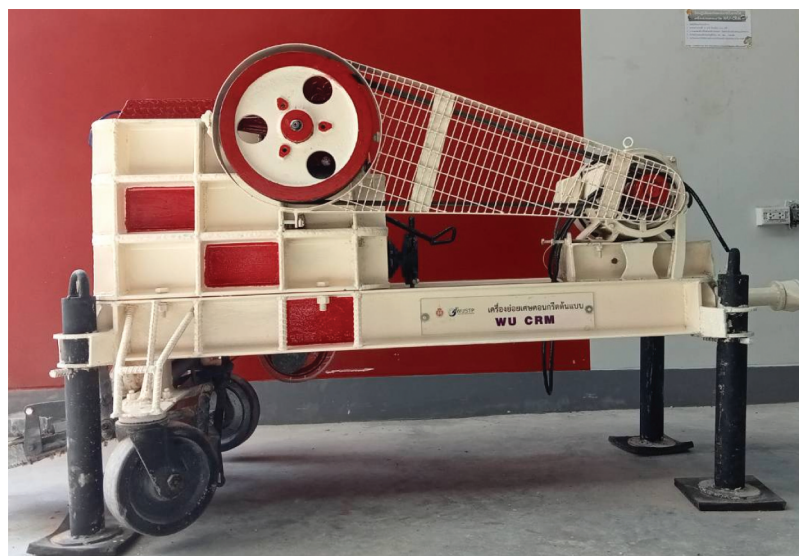
Figure 5. Crusher machine used for concrete crushing.
