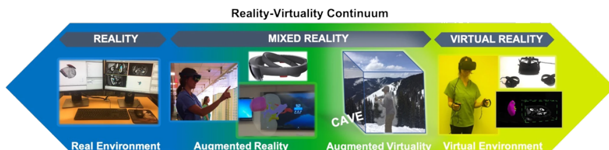
Figure 1.1: Milgram's Reality-virtuality Continuum about Real Environment, Augmented Reality, Augmented Virtuality and Virtual Reality [299]
