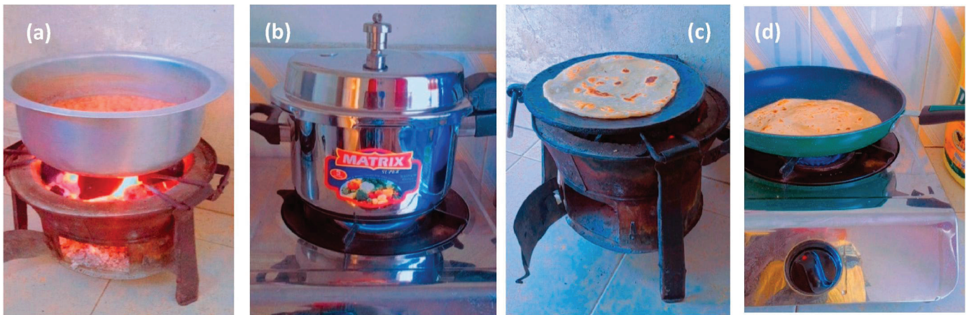
Fig. 8. Pans used in the Kenya Interventions study. (a): traditional sufuria boiling beans on a charcoal stove. (b) pressure cooker preparing beans on an LPG stove. (c) traditional frying pan preparing chapatis on a charcoal stove and (d) frying pan preparing chapatis on LPG stove. Photo credit: Paulah Okoth
