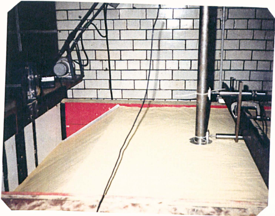
Plate 7.6 Arrangement for pile test in a slope terrain
