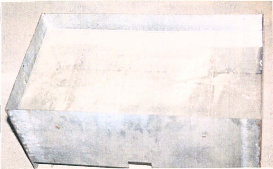
Plate 6.6 Baffle used for sand raining in preparation of loose packing
