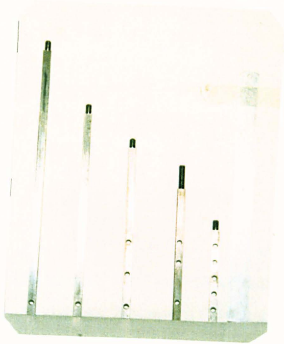
Plate 5.3 Square pulling arm for centrifugal test
