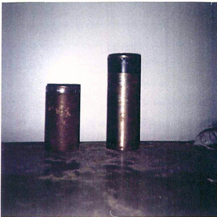
Plate 5.2 Single cylindrical pile used in conventional test
