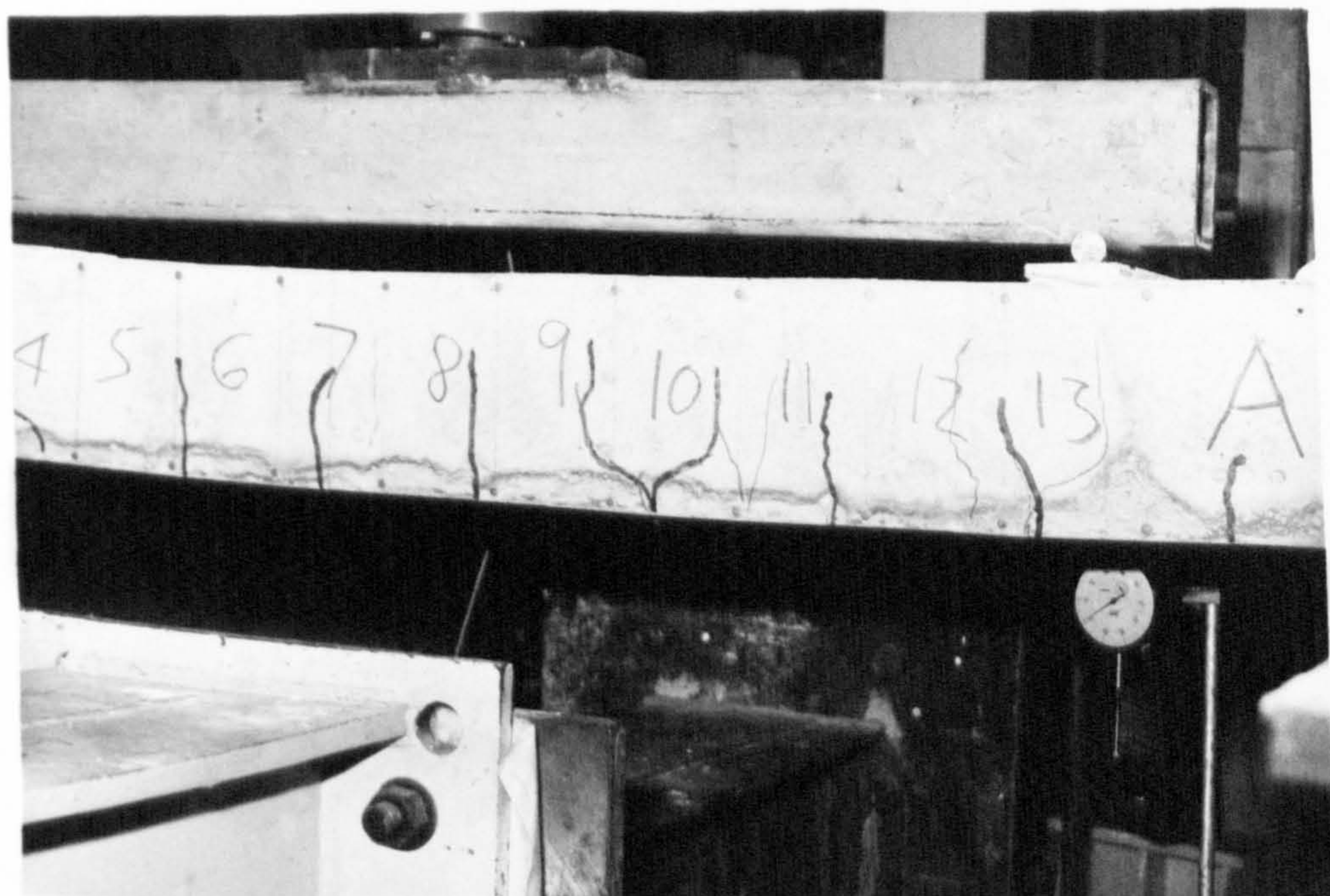
PLATE 3 Crack Pattern on Elevation
