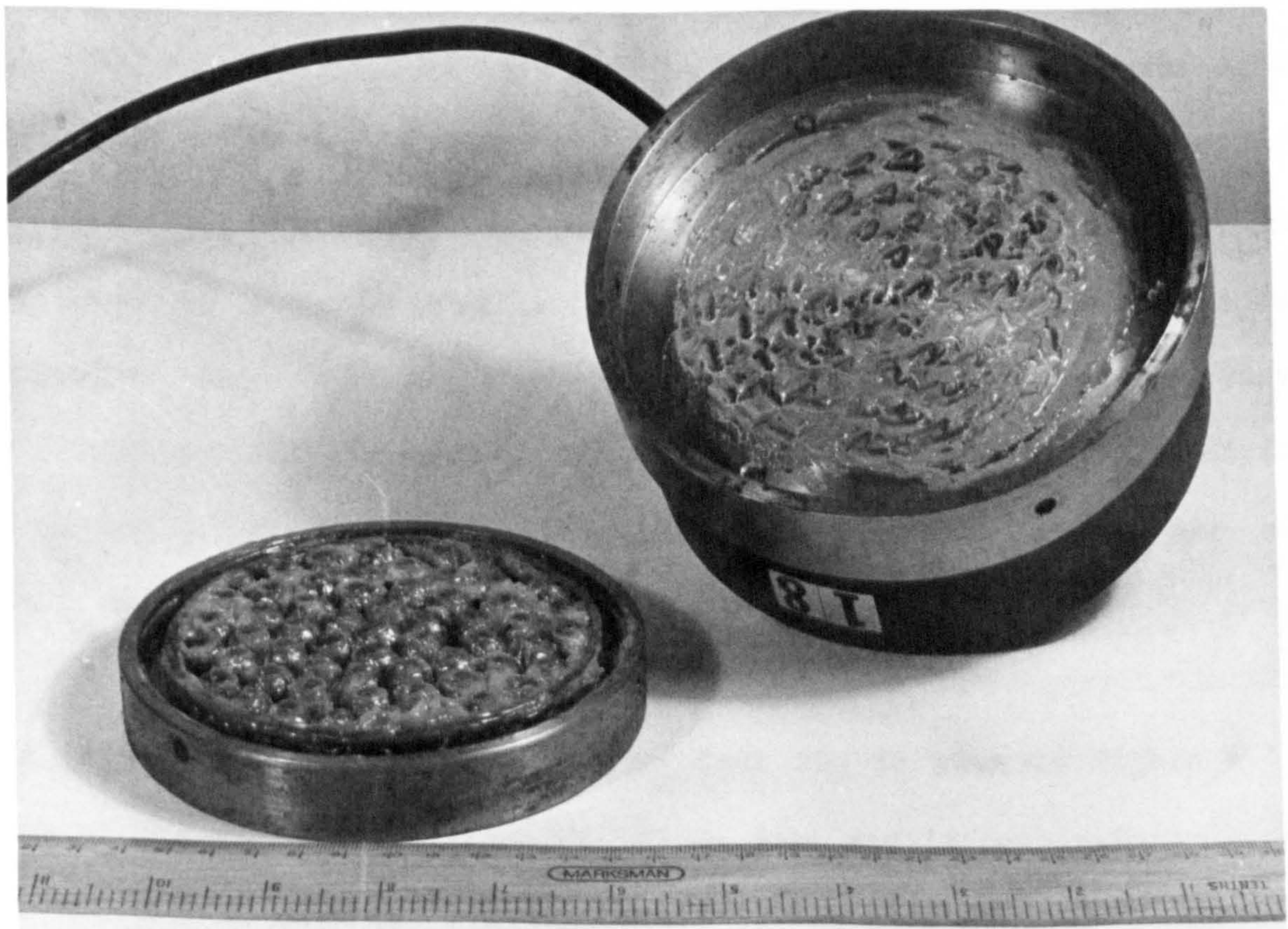
PLATE 3.7 MODEL DECK SUPPORT, WHICH INCORPORATED A LOAD CELL AND A BALL BEARING UNIT, AND ALLOWED MOVEMENT IN THE X-Y PLANE.
