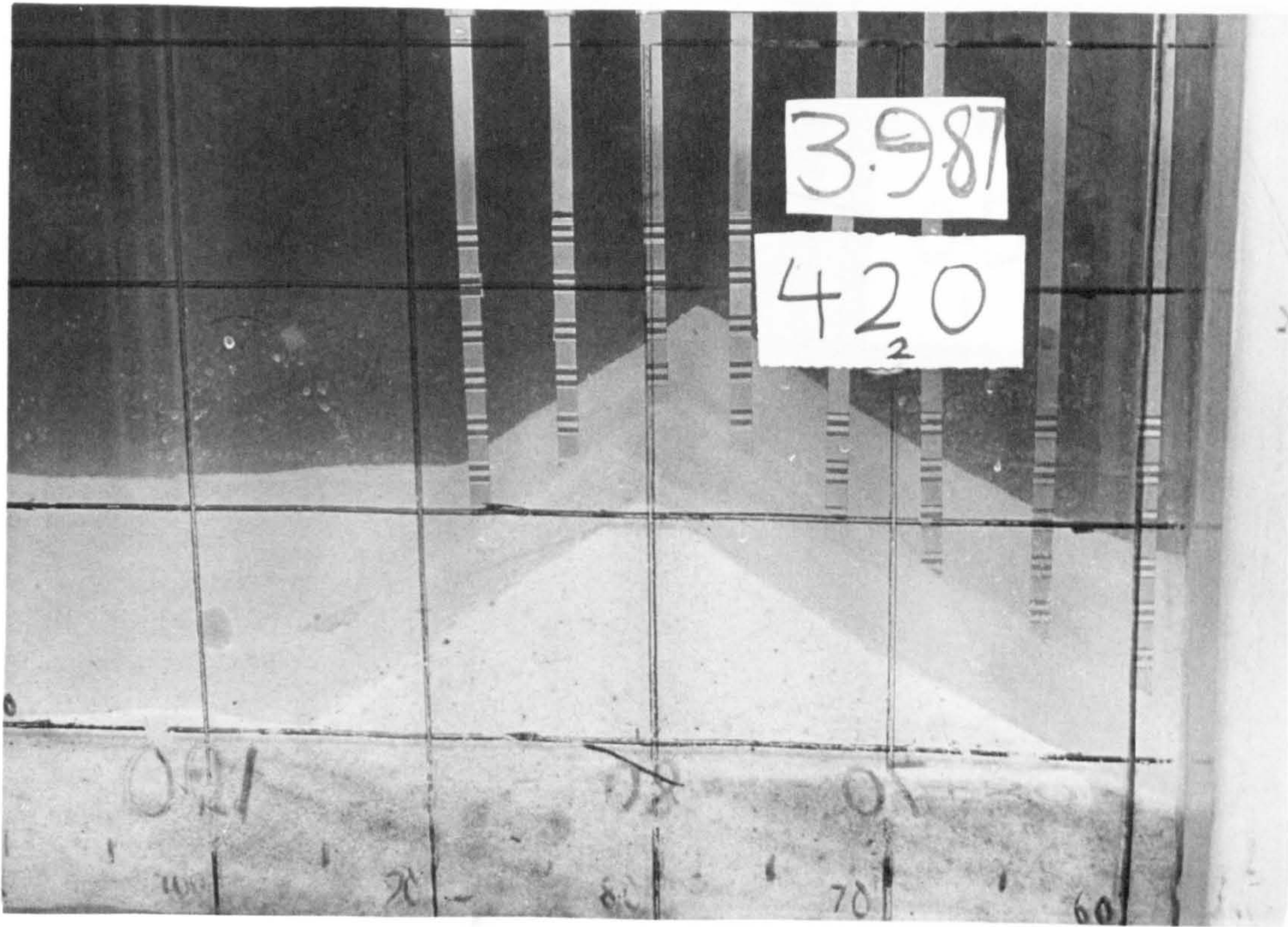
Plate 6.6 Lee of the dune (equal to the angle of repose of sand)
