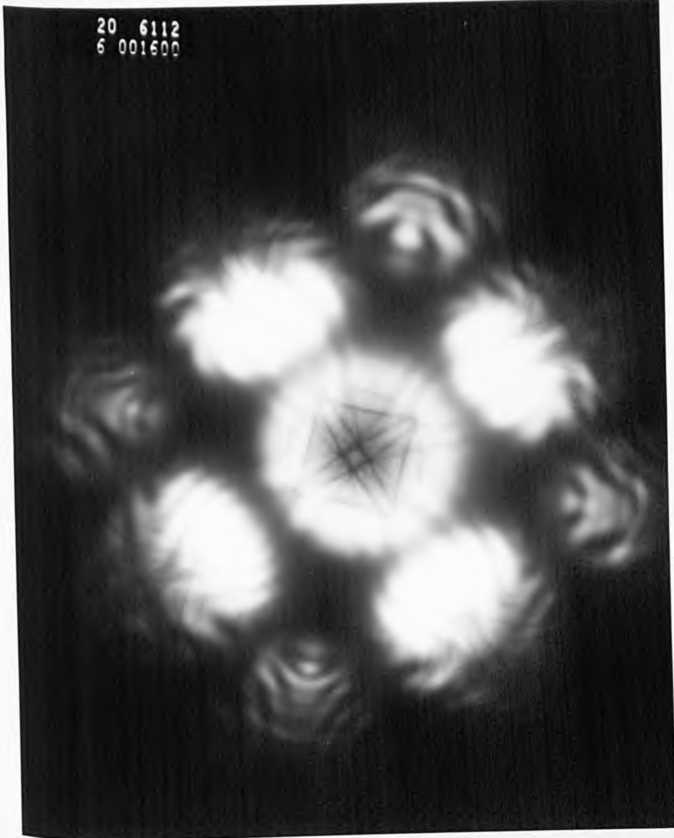
Fig. 3.12(a). The [001] LACBED pattern was taken from a germanium single crystal (120Kv).
