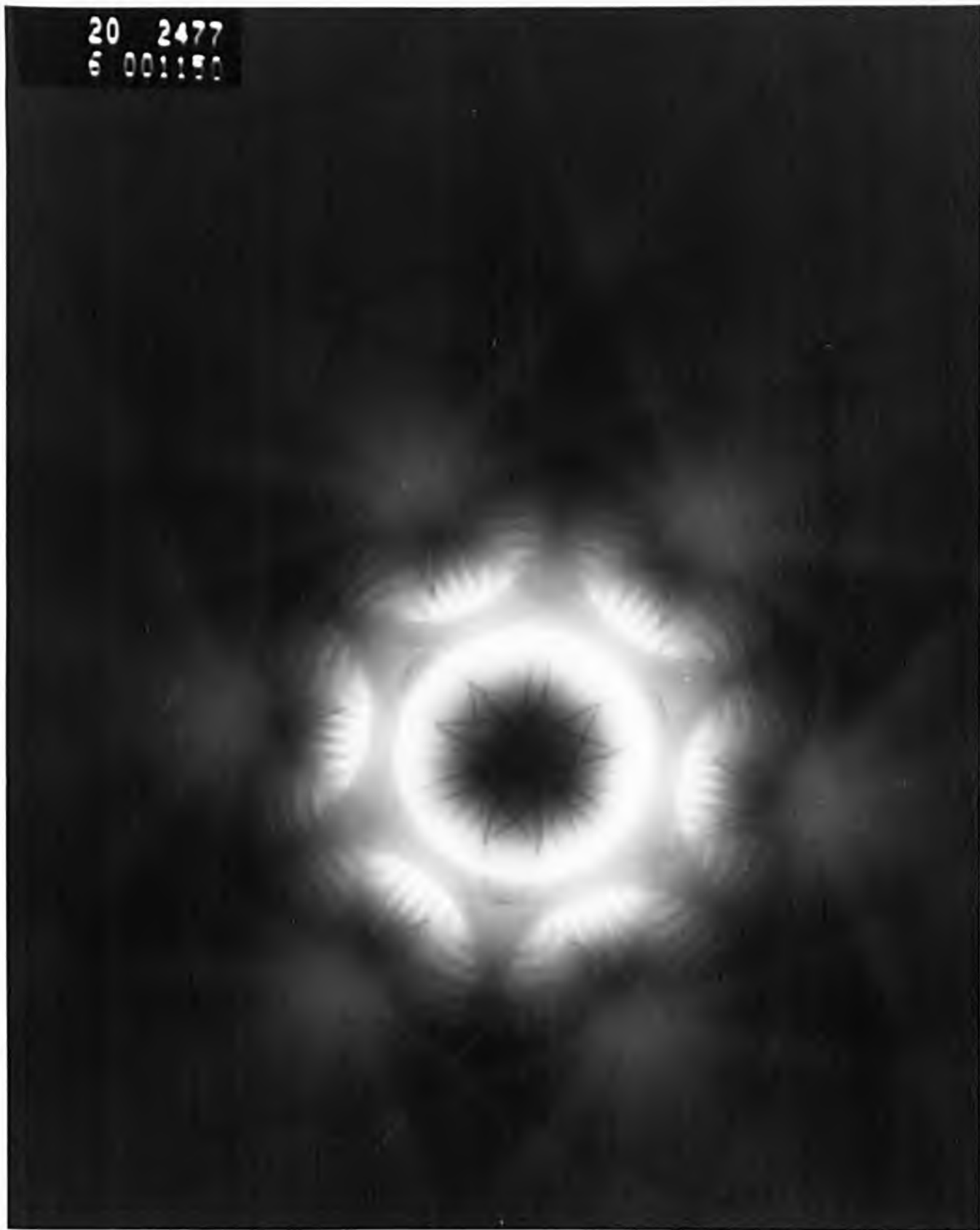
Fig. 3.10. The [111] CBED pattern was taken from a germanium single crystal (120Kv). The central disc is 000 type and the next discs around the centre are of the type 220.
