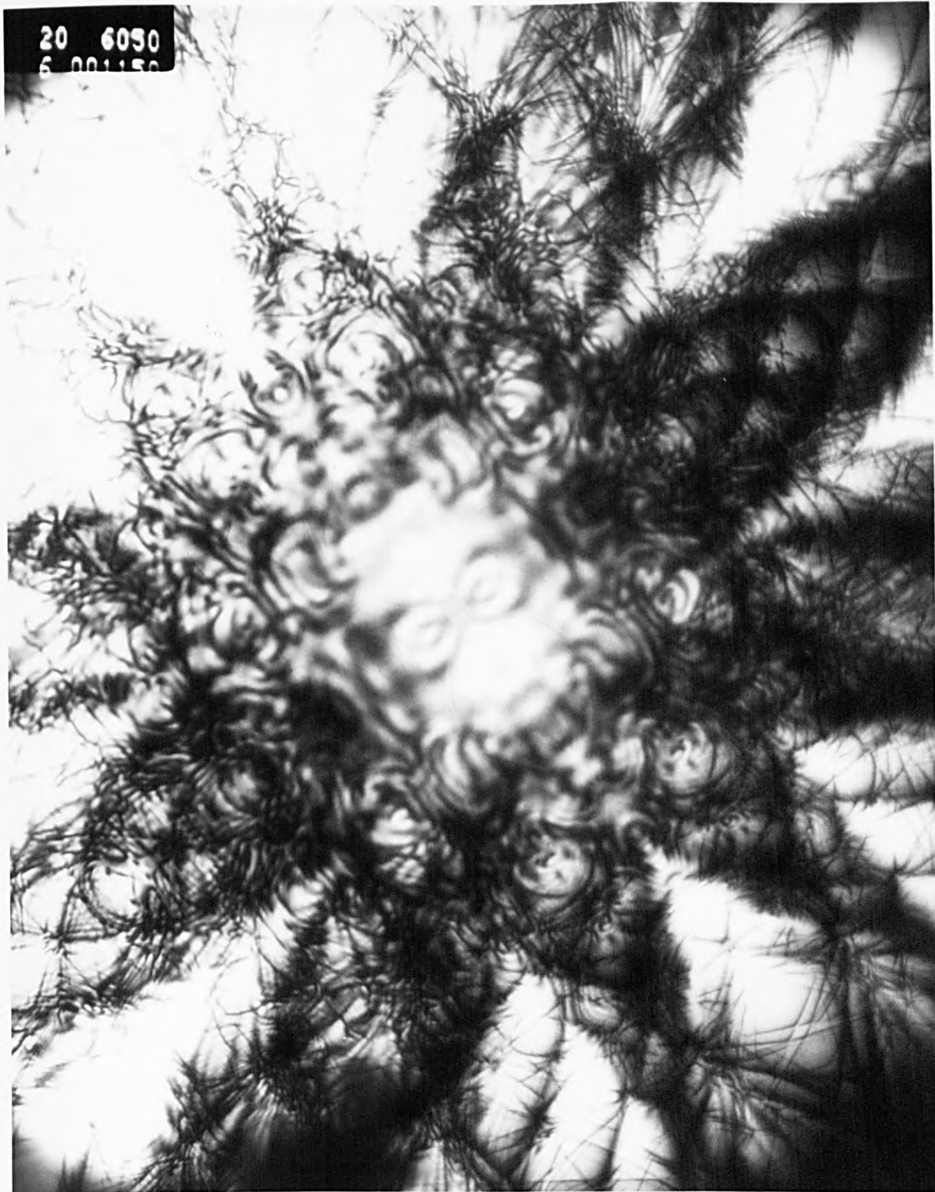
Fig. 3.12(b). The [011] LACBED pattern was taken from a germanium single crystal (120Kv).
