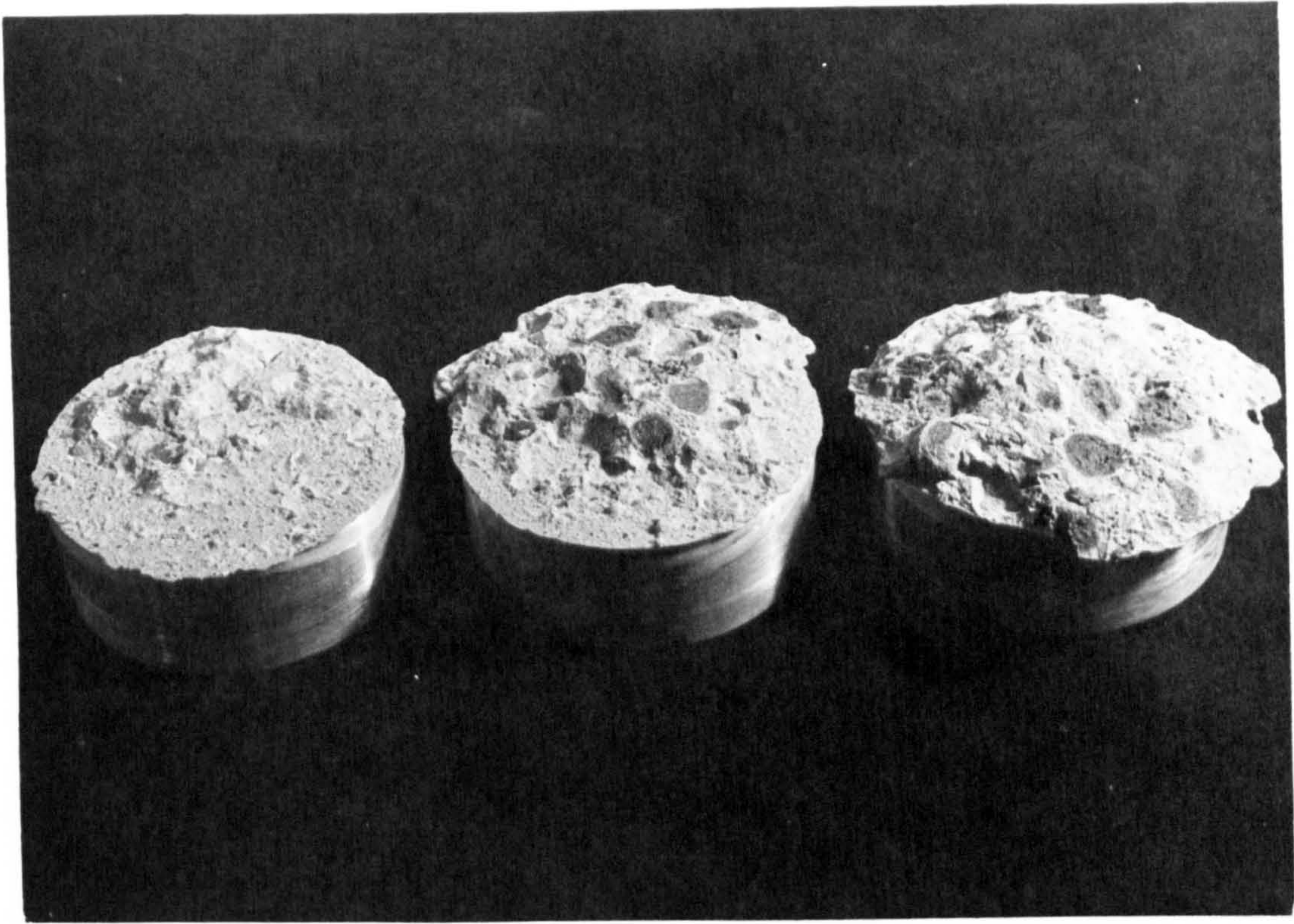
Figure 6.82a: Typical failures from surface pull off tests on fully Lytag concretes, showing variation in the failure depth
