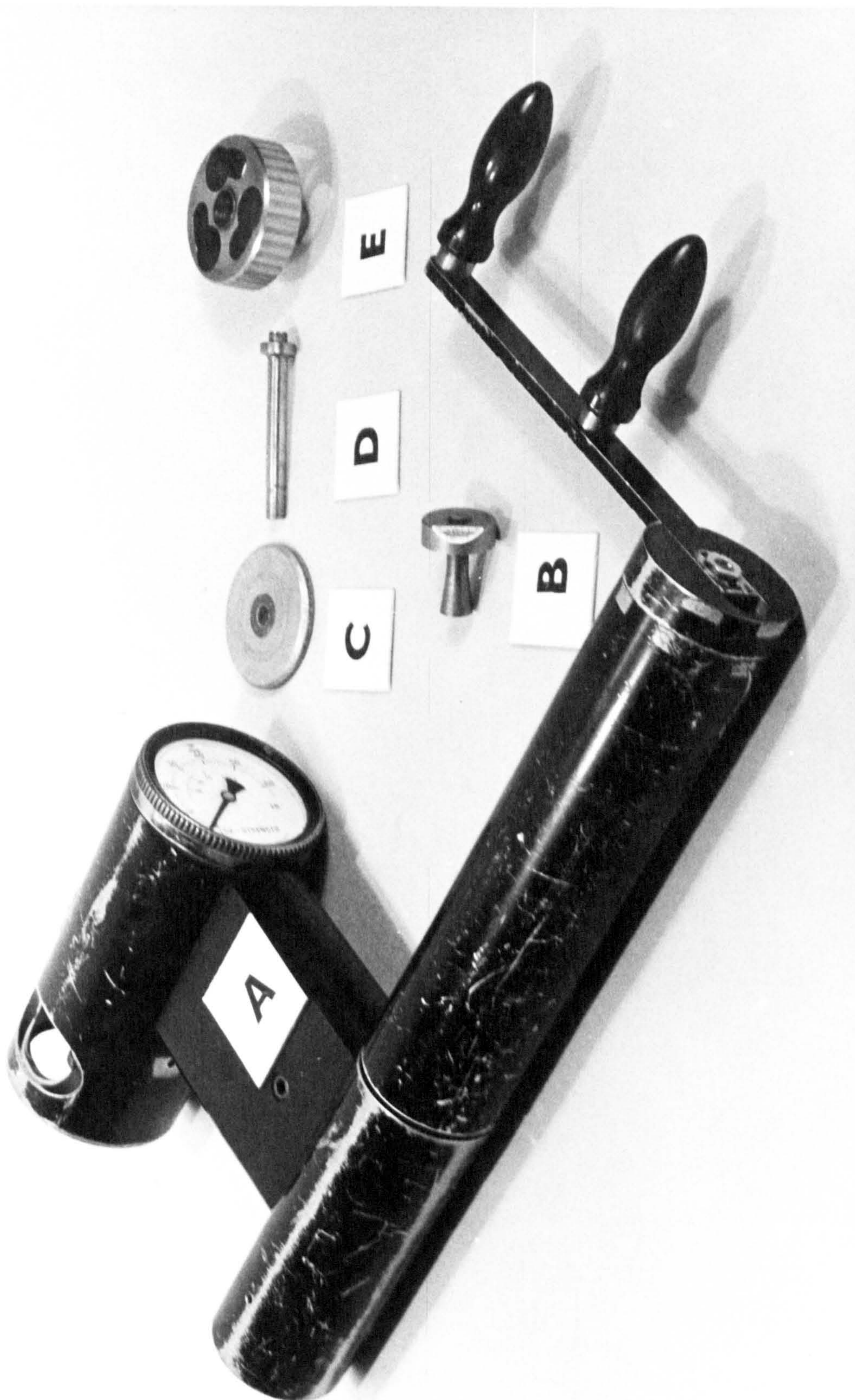
A: Lok-Test instrument; B: Lok insert; C: centering plate; D: pull bolt; E: coupling
