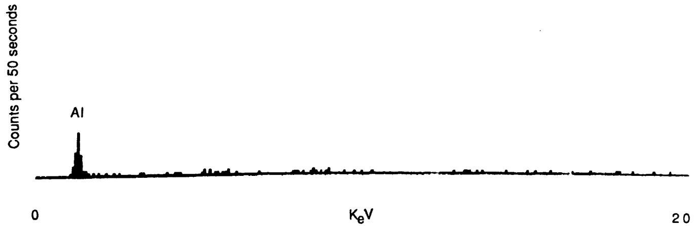
Fig. 3.13.a. Control. Paneth cell of rat small intestine. X-ray emission spectra of the apical cytoplasm of the homogenous oval electron dense granules. The aluminium (Al) peak was derived from the grid material.
