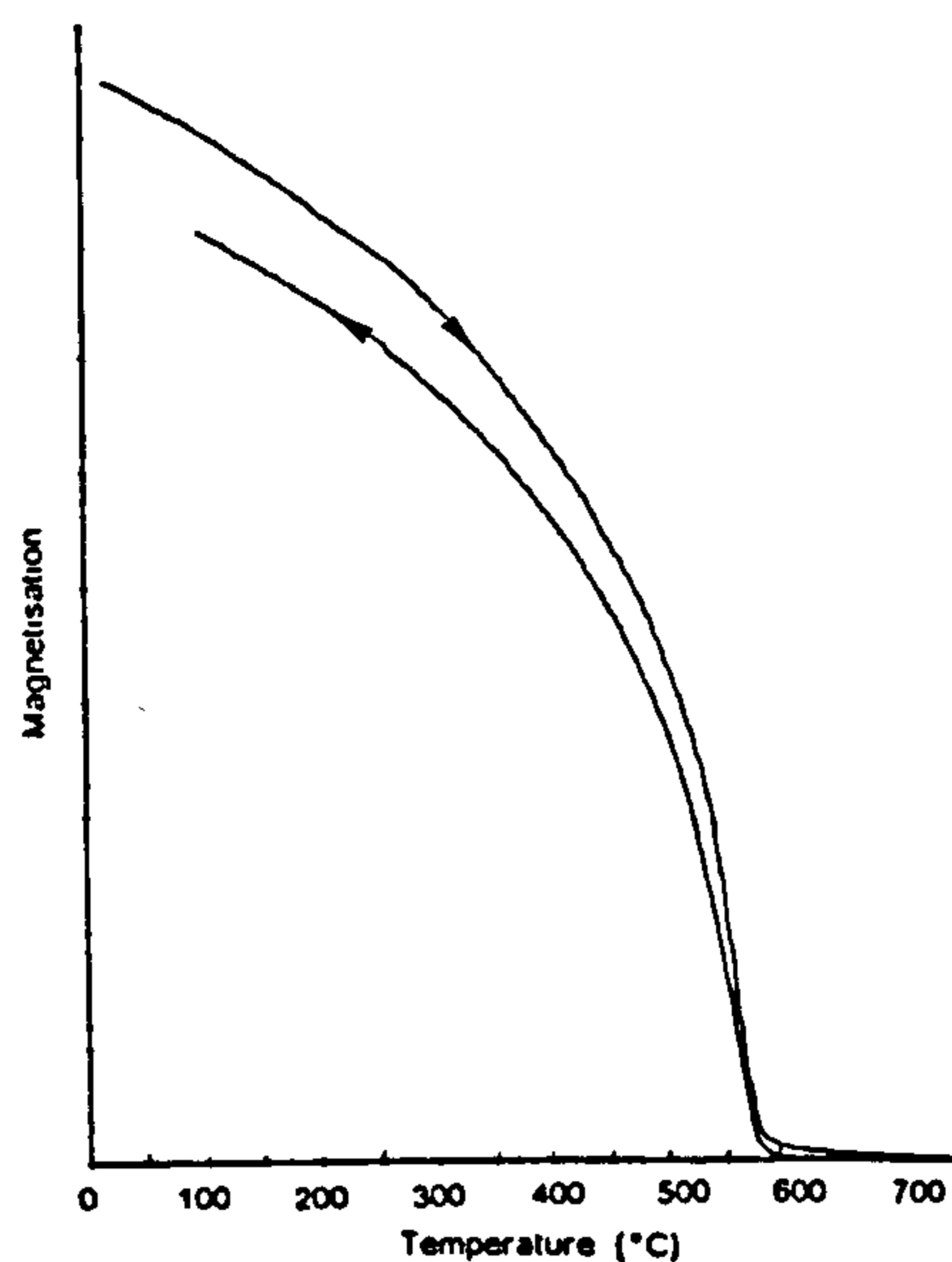
Figure 3.2. The thermomagnetic behaviour of synthetic magnetite measured using the system described. The Curie point temperature is 575°C on heating and 582°C on cooling.
