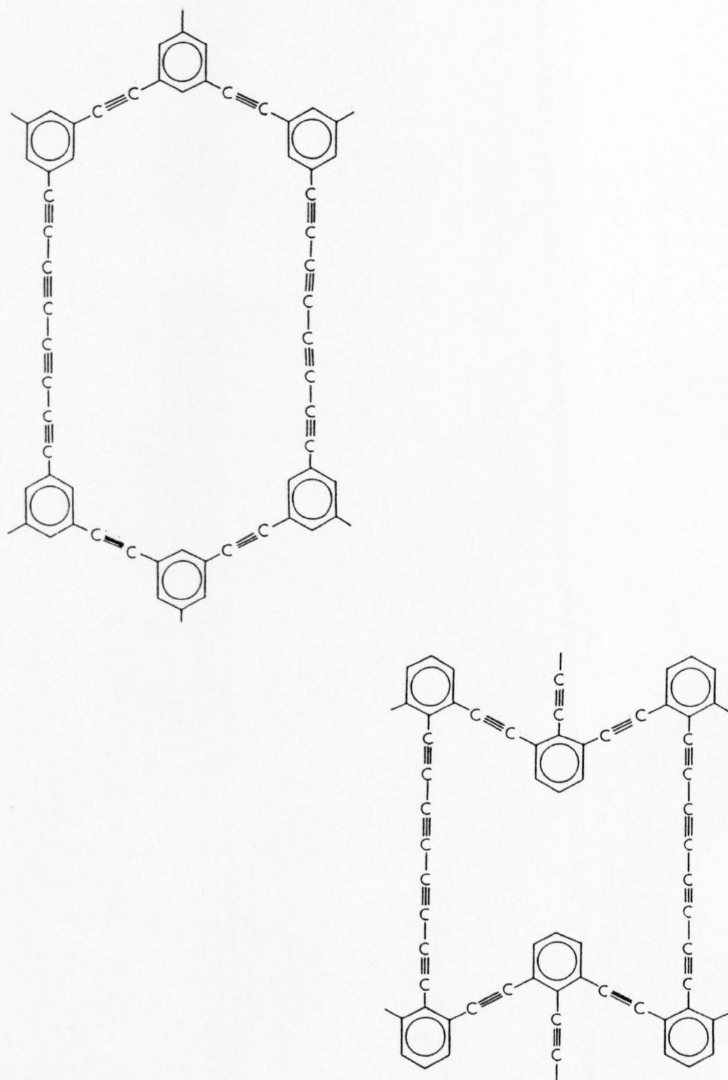
Fig.8.10 Two of the theoretical molecular structures investigated by Nkansah et al. (1994). The structures are termed 1,4 flexyne (top), 1,4 reflexyne (bottom) where the numerals refer to the number of C\equiv C bonds.
