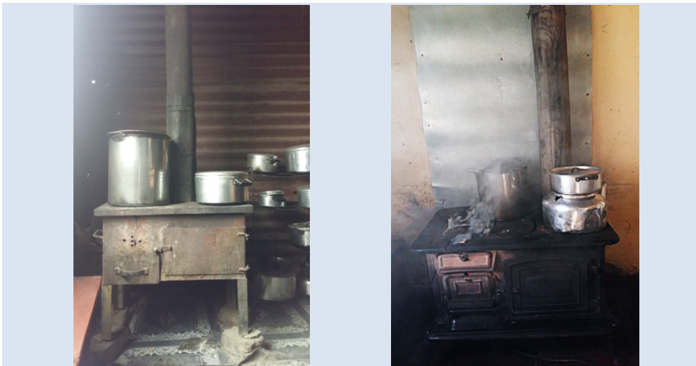
Photo 15: Self-fabricated welded stove. Source: Fieldwork, 2017, Wesselton township
