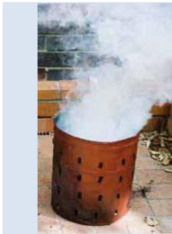
Figure 12: Imbaula stove using the traditional bottom-up ignition method
