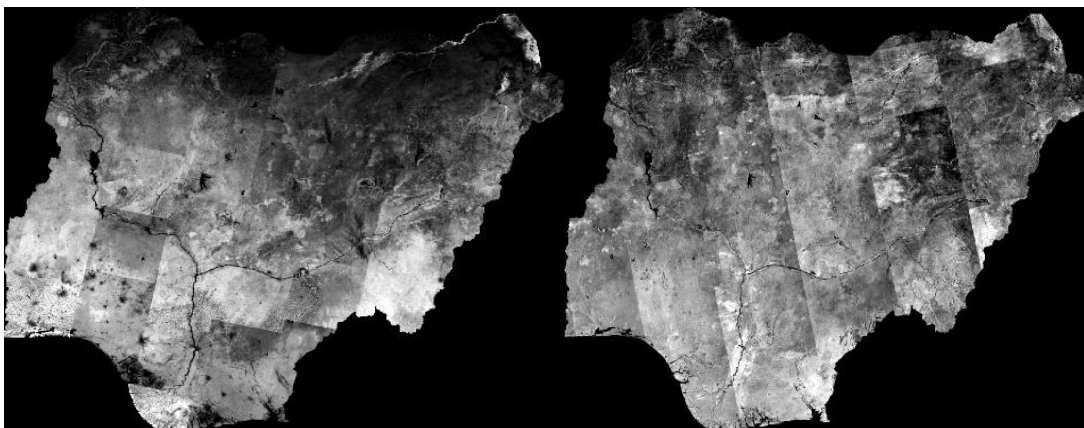
Figure 5.4: NDVI from the optical bands (left) and DPSVI from the VV and VH radar bands (right)
