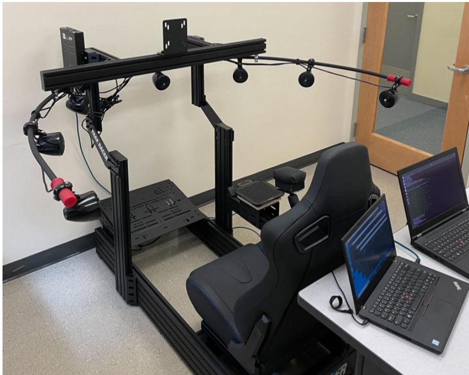
Figure 5. Nonvisual control interface using spatialized audio, gestural interaction, and haptics.
