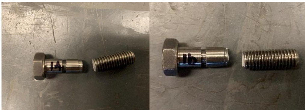
Figure 49. Bolt 1A (left) and Bolt 1B (right) after testing (both titanium bolts).
