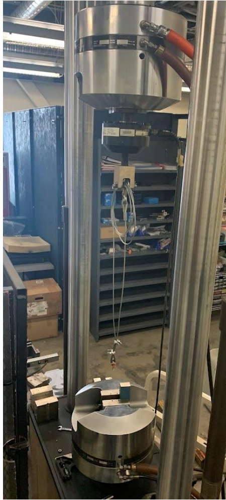
Figure 37. MTS 810 servo-hydraulic machine with a 22kip load cell at the University of Maine Advanced Manufacturing Center.
