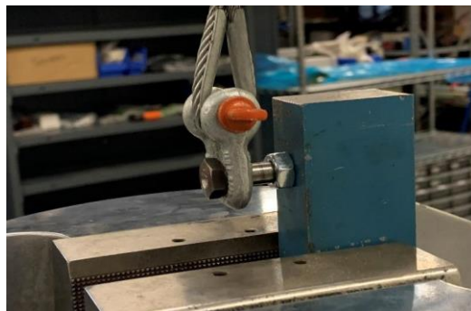
Figure 38. Bolt in the custom fixture with a nut threaded on for additional stability, with a braided steel cable clamped to the bolt via a shackle.
