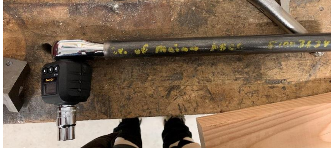
Figure 39. Breaker bar, 13mm socket, and a half-inch drive socket attached to a digital torque wrench.
