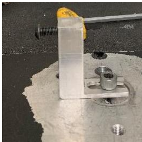
Figure 36. Custom bending fixture for use with an Instron 8872.
