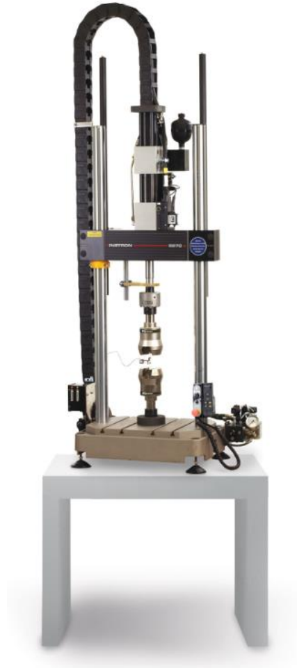
Figure 35. Instron 8872 servo hydraulic machine.
