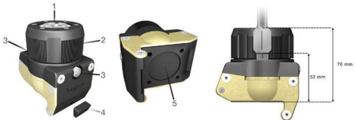
Figure 14. OPRA Axor II standard mounting mechanism, including (1) jaws for abutment connection, (2) rotatable grip for attachment and detachment, (3) alignment nuts, (4) plug for adjustable screw access, and (5) standardized prosthetic attachment area. Ref[59].
