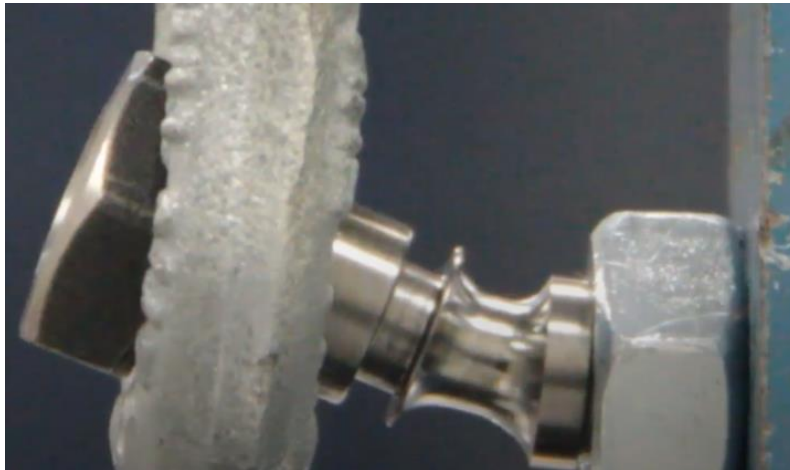
Figure 54. Display of plastic yielding in bolt during testing.
