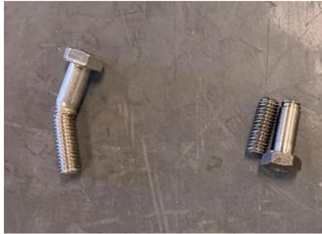
Figure 48. Unmodified steel bolt (left) and unmodified titanium bolt (right) after testing.
