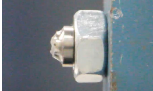
Figure 52. An example of a bolt that sheared at its notch region.
