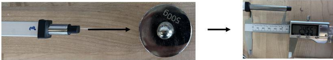
Figure 4.16. Method flow diagram used in the software timed distance measurement experiment where the actuator distance of the actuator pushing a known load is measured.
