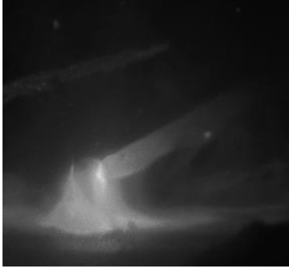
Figure 6.17 Examples of the mixed mode in DE-GMAW.
