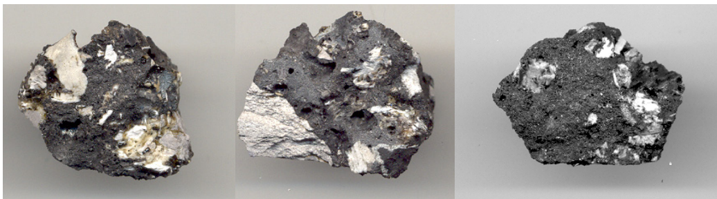
Figure 5: Clinker fragments highlighting rock fragments (light colour) in a matrix of “glass” (black).
