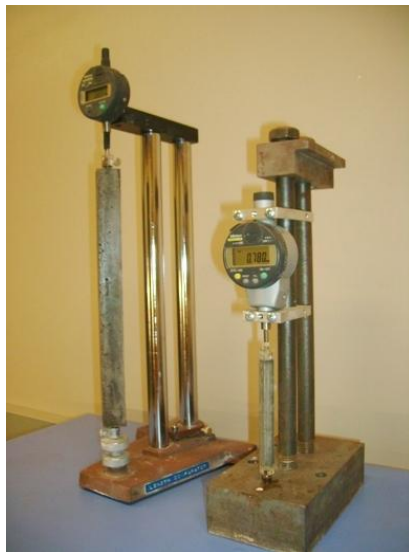
Figure 4. Measurement of specimens using two separate digital gages for standard size (left) and modified size (right) specimens
