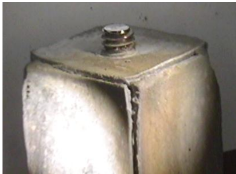
Figure 8. Diagonal cracks along all edges for a standard size specimen, wider cracks are observed along the edges
